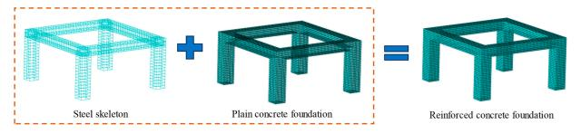
Figure 11. Schematic diagram of the numerical model of the reinforced transmission tower foundation.
