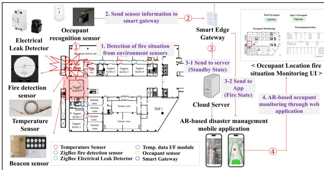
Figure 13. SFSMS mobile/web application data flow.
