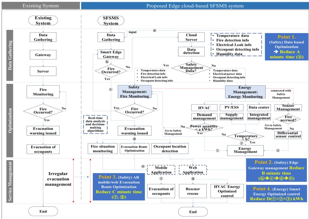
Figure 18. SFSMS algorithm compared to the existing system.
