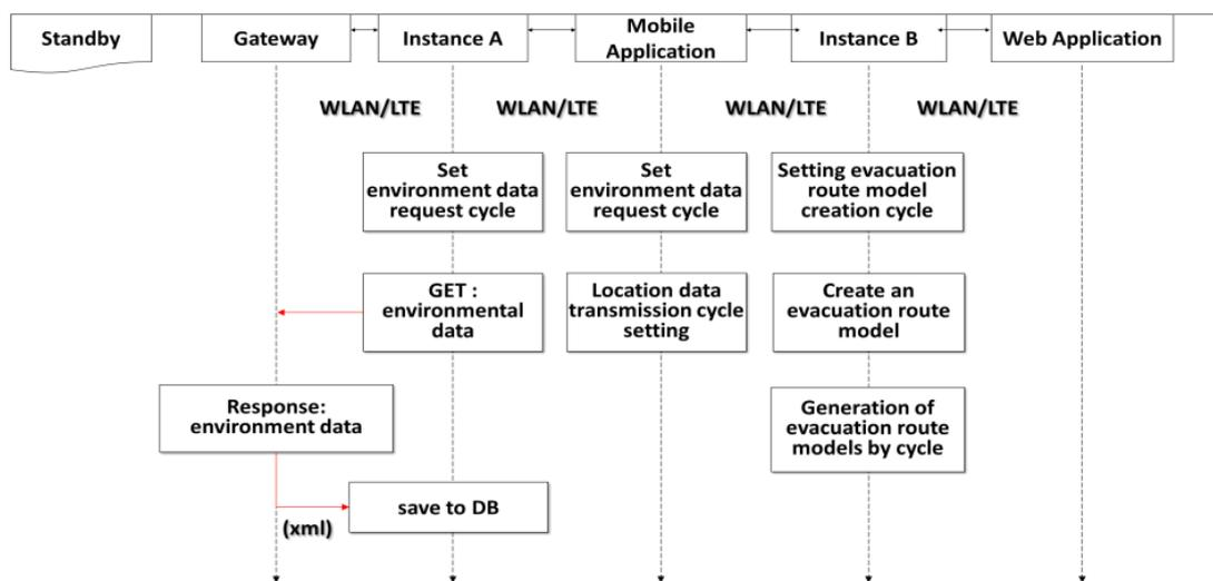
Figure 9. System state: standby data flow.
