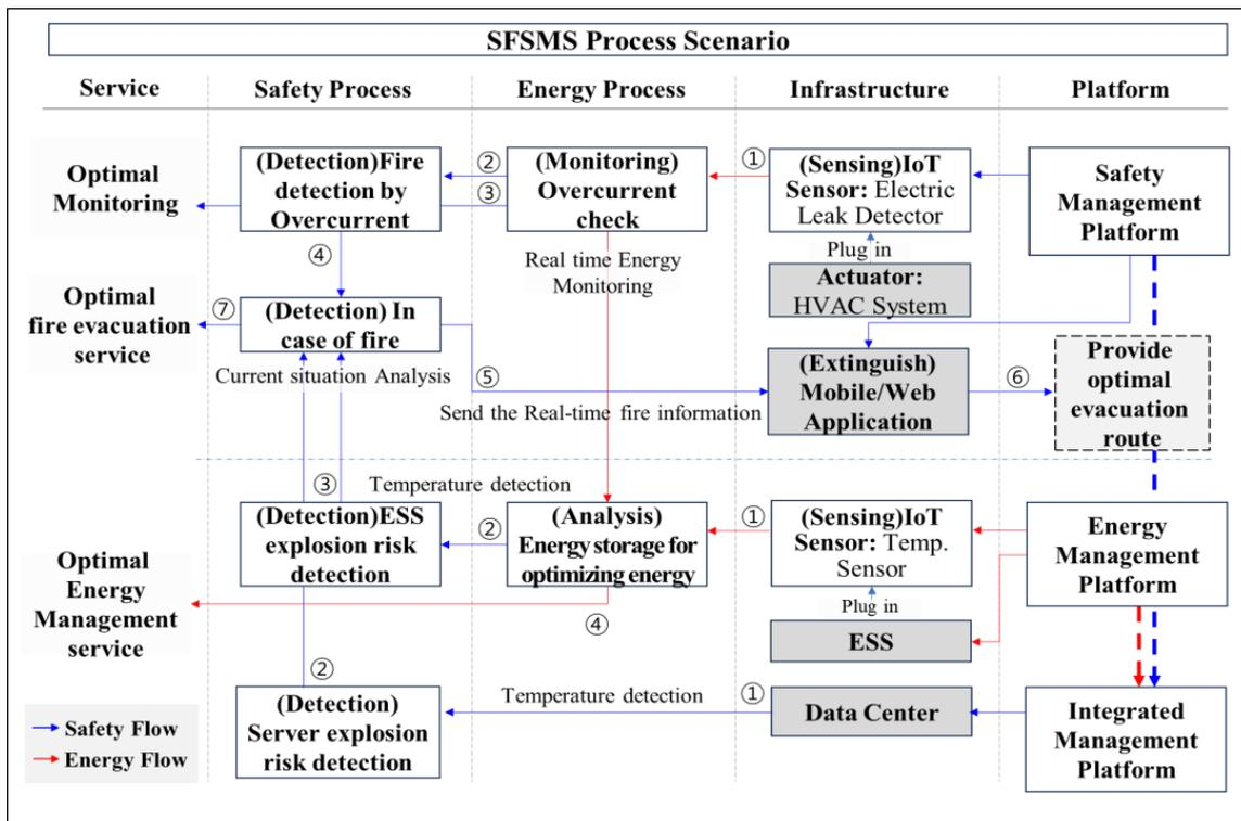
Figure 17. Safety and energy management control process scenario in SFSMS.
