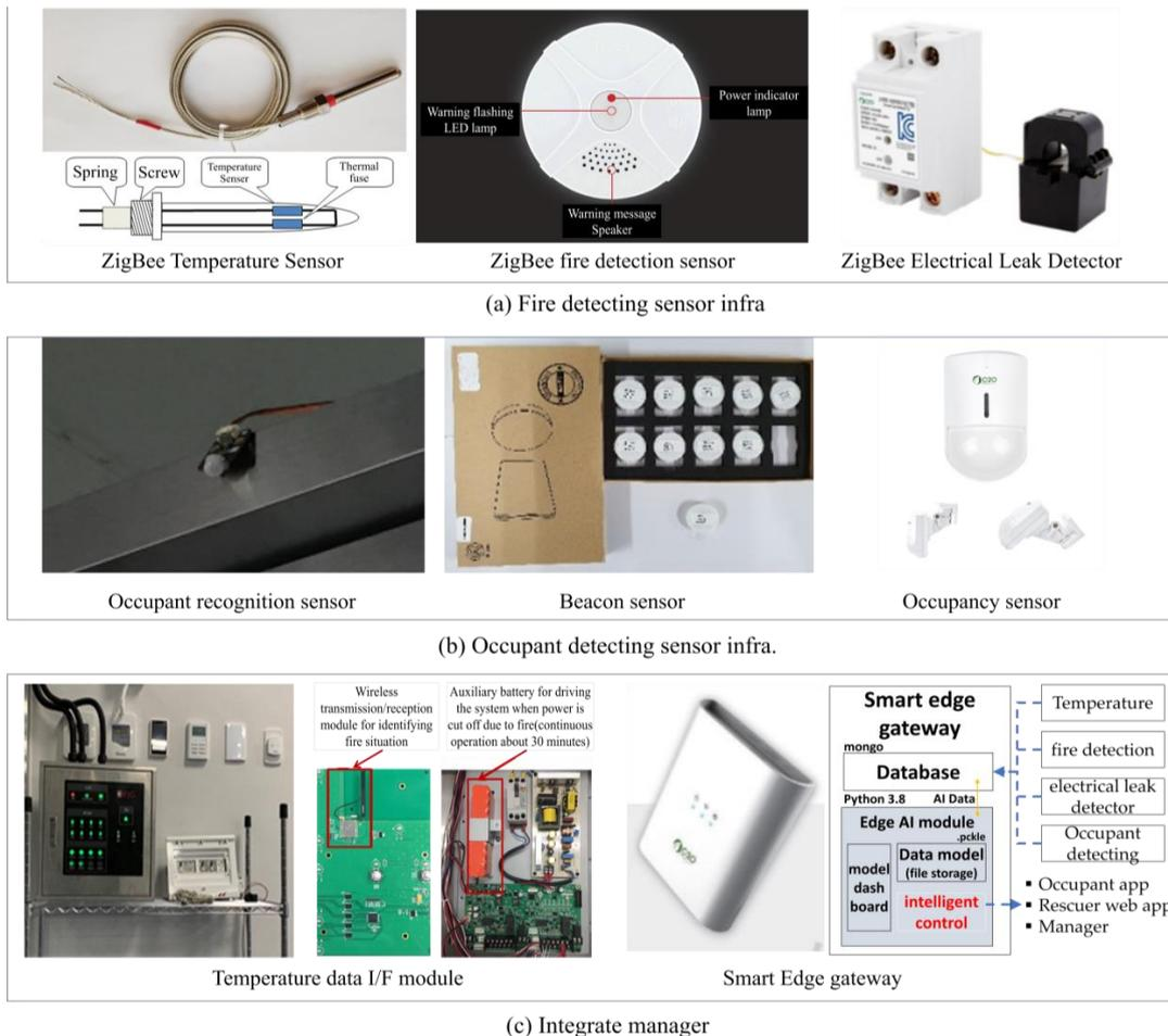
**Figure 7.** Fire detection sensors.
