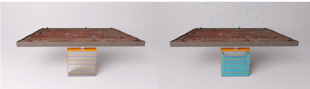
**Figure 7.** Visualization of the extensive green roof before and after the simulation. The total accumulated amount of runoff water to the stormwater tank is  $7.25 \text{ m}^3$ .
