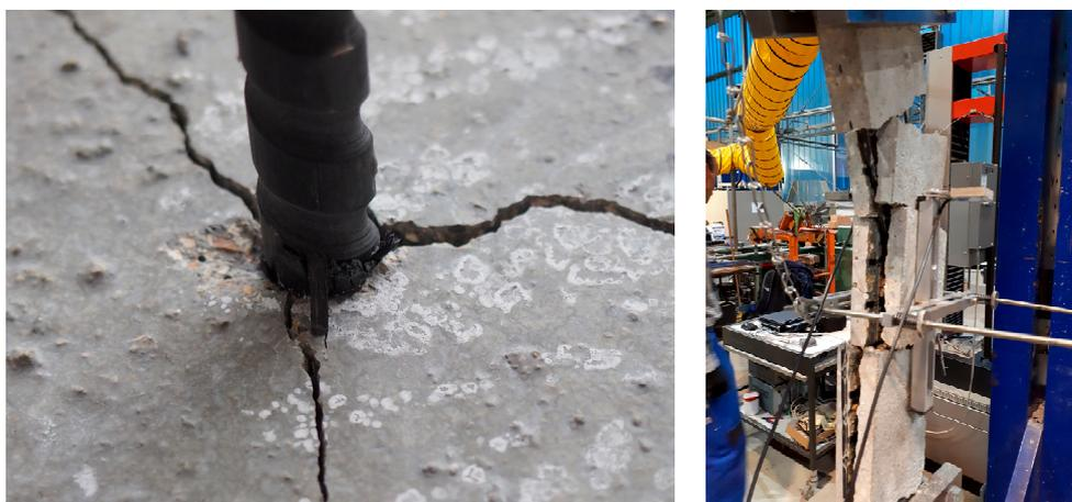
Figure 12. Splitting forces of carbon reinforcements; left: rebar; right: carbon grid (photo: S. May).
