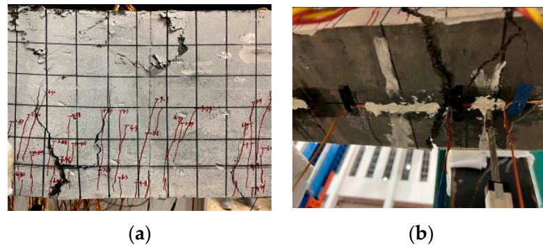
Figure 9. Failure and crack distribution of PSRUHPC beam: (a) crushed UHPC; (b) three main cracks in the tension zone.
