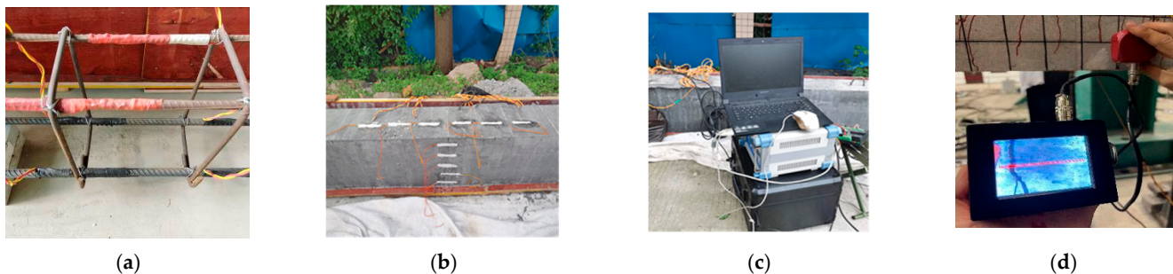
Figure 6. Main test equipment: (a) steel bar strain measuring point; (b) UHPC strain gauge points; (c) unbonded prestress incremental measurement; (d) crack width measurement device.
