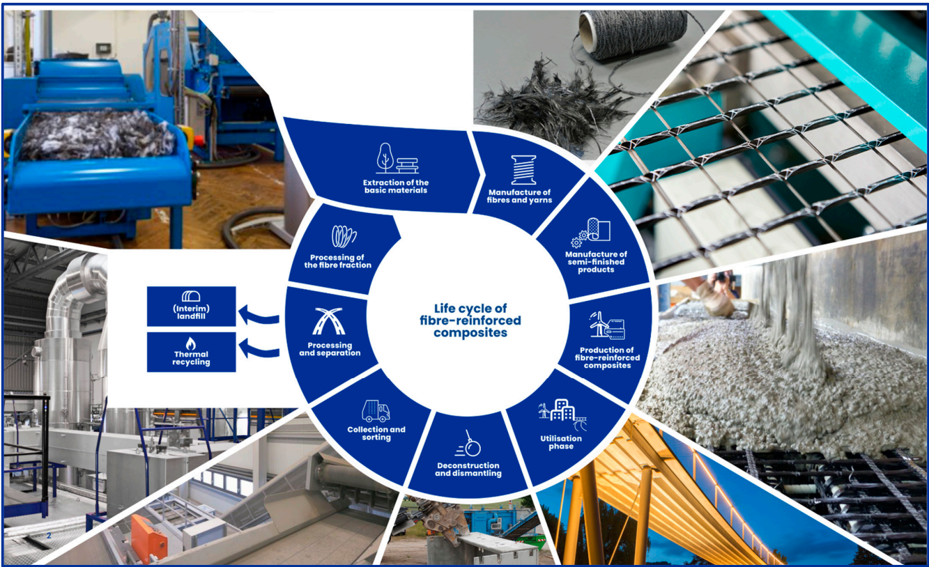
Figure 4. Phases of the material cycle of carbon concrete including examples of technological availability, © C 3 Verband.
