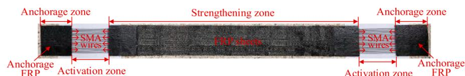
**Figure 11.** SMA/CFRP composite pre-stressed strengthening system, reproduced with permission from [77], Elsevier, 2023.
