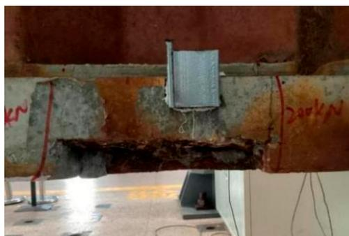
**Figure 20.** Concrete spalling of Beam A2 during loading process.
