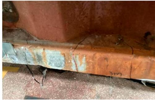
**Figure 18.** Development of cracks of Beam A2 when the load is 200 kN.
