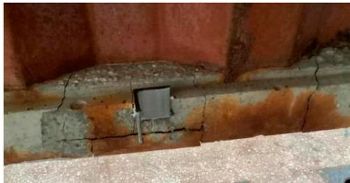
**Figure 19.** Development of cracks on Beam A2 when the load is 235 kN.
