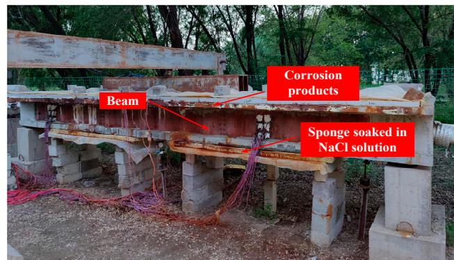
**Figure 4.** Arrangement of accelerated corrosion test.
