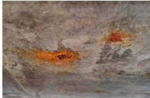
**Figure 12.** Corrosion of the bottom plate of Beam A2 on the 30th day of the accelerated corrosion test.
