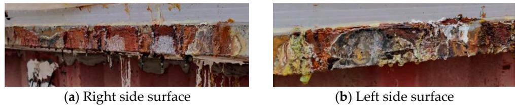
**Figure 11.** Corrosion products on the side surfaces of Beam A2 on the 30th day of the accelerated corrosion test.
