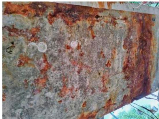
**Figure 15.** Corrosion-induced cracks on the bottom plate of Beam A2 on the 100th day of the accelerated corrosion test.
