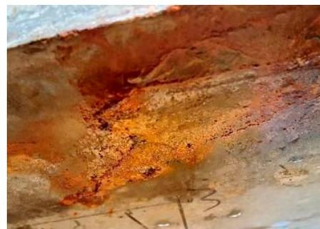
(b) Corrosion products on the bottom plate
