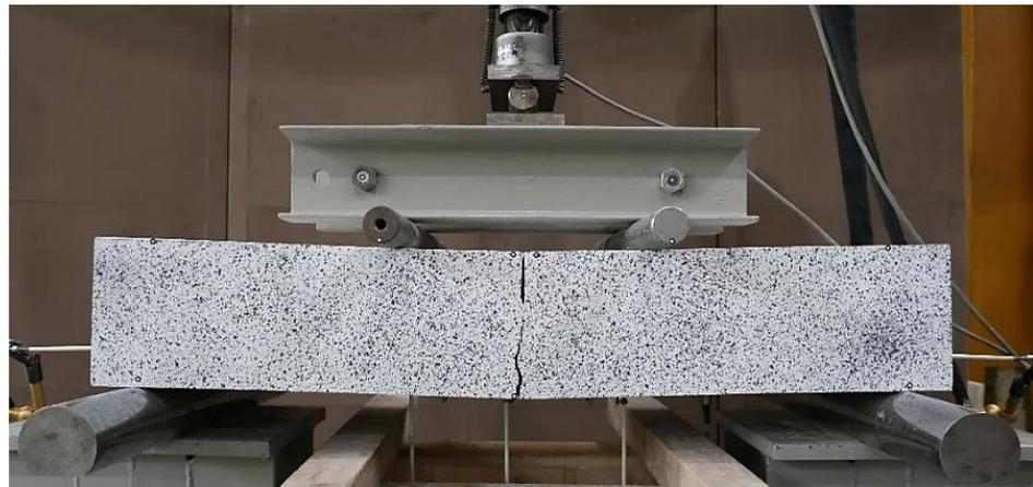
**Figure 10.** Beam subjected to four-point bending test according to RILEM RC5 with some specific modifications. Beam dimensions are  $L \times B \times D = 1000 \text{ mm} \times 340 \text{ mm} \times 170 \text{ mm}$ .
