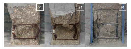
Figure 7. Specimens S1, S2, and S3 failure modes—bottom view of the beam's critical zone.
