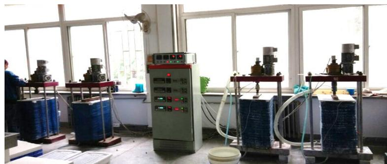
**Figure 1.** Test device for sulfate attack of concrete under drying–wetting cycles coupled with alternating loads.
