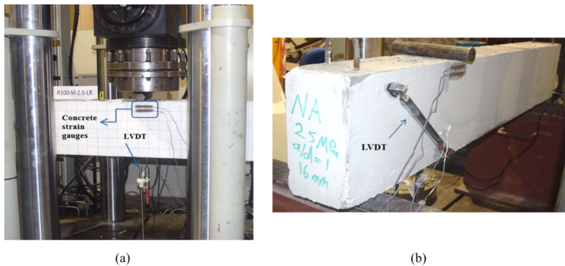
Figure 4. Instrumentation of the specimen: (a) strain gauges on concrete and vertical LVDT, (b) diagonally mounted LVDT.
