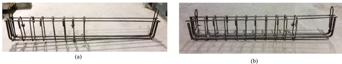
Figure 2. Steel reinforcement steel cage: (a) a/d = 2.5 , (b) a/d = 1.15 .
