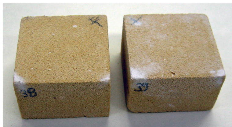
Figure 9. White haze formation on Maastricht limestone after 6 applications of CaLoSiL IP25.
