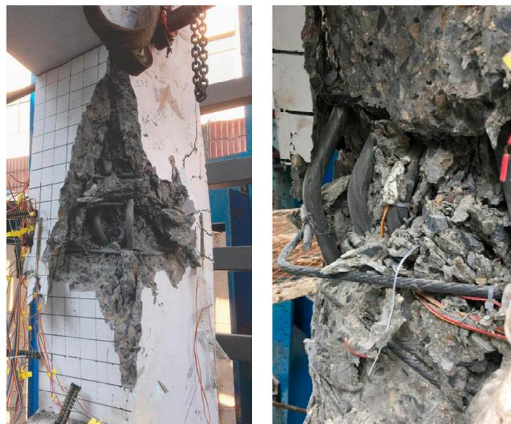
**Figure 8.** Compression resulting in local buckling of NPR735 rebars in specimen BZ-1.
