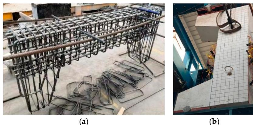
**Figure 2.** Construction process of the specimens: (a) skeleton of steel reinforcement, (b) finished concrete column.
