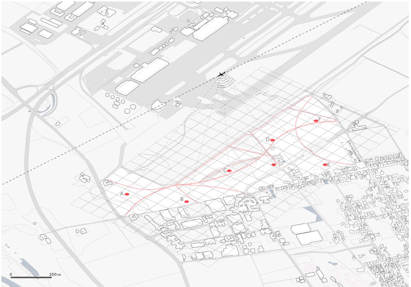
**Figure 10.** The site model was overlaid with a supporting grid for defining simulation areas. The listener was positioned at six points along the grid (marked A–F). Map by the students of the ‘Precision Landscapes’ seminar (TUM, 2022).
