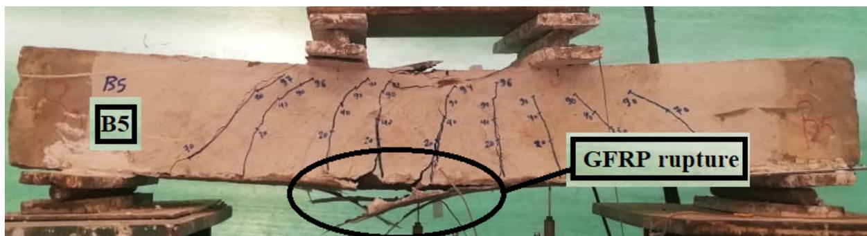
Figure 15. The final crack of beam B5-0.6-EP.
