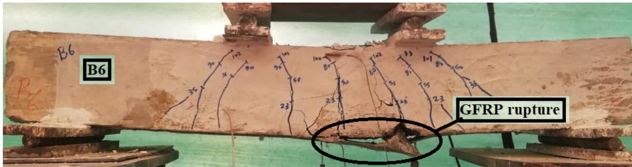
**Figure 16.** The final crack of beam B6-1.2-EP.
