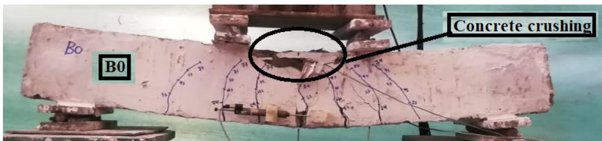
**Figure 10.** The final crack of beam B0-Control.
