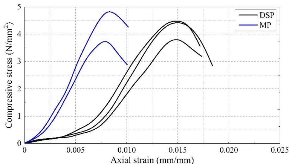
**Figure 8.** Stress–strain curves in compression of the prisms with dry stack (DSP) and mortar joints (MP).
