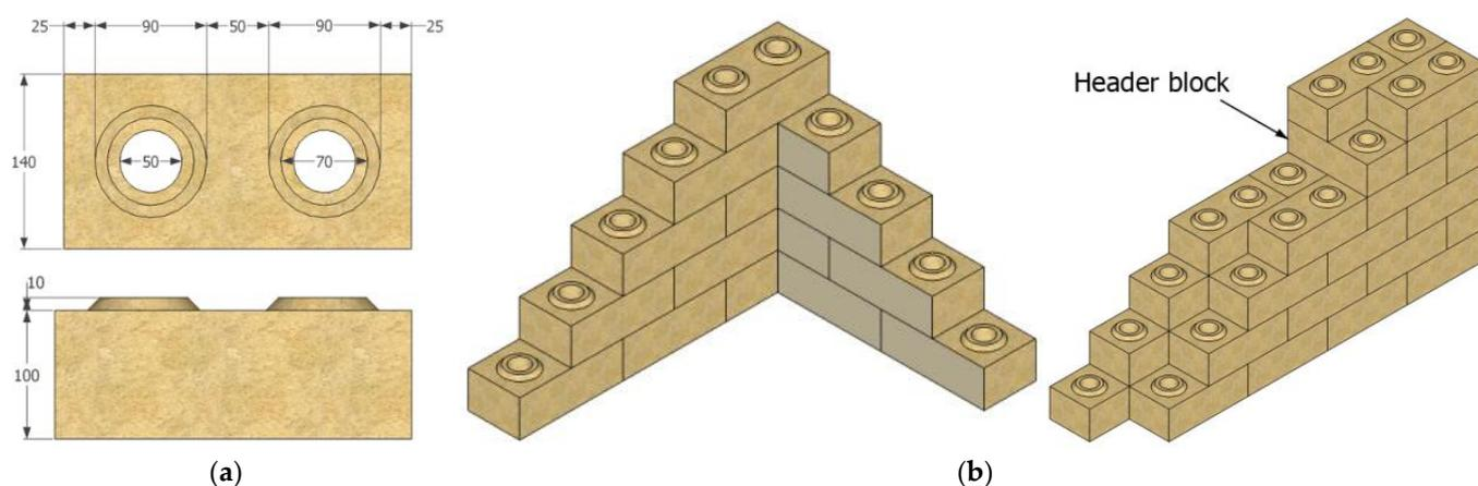
**Figure 4.** Building system adopted for the experimental program [45]: (a) geometry of the iCEBs and (b) running bond pattern for single-leaf and double-leaf walls.
