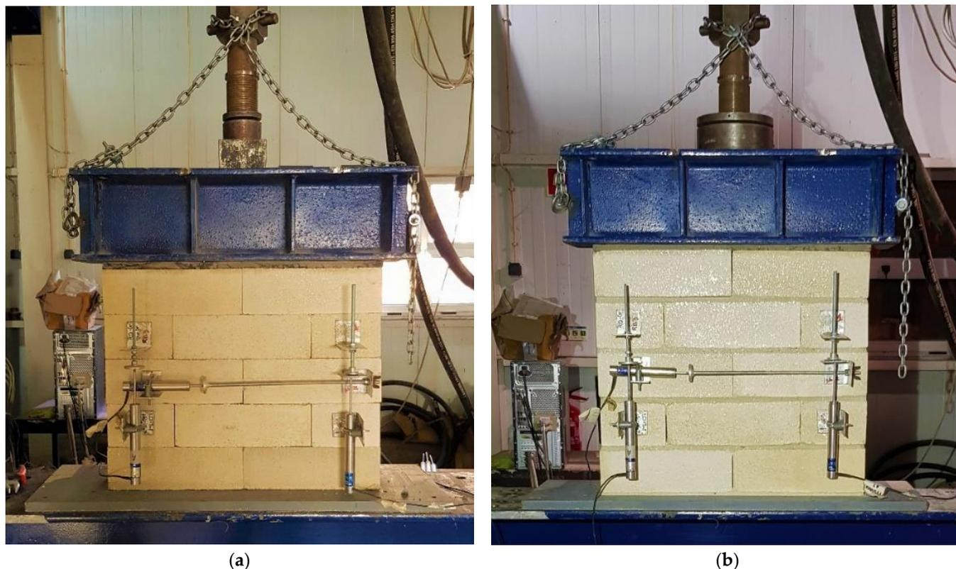
**Figure 7.** Setup of the compression tests conducted on masonry wallettes: (a) DSW and (b) MW.
