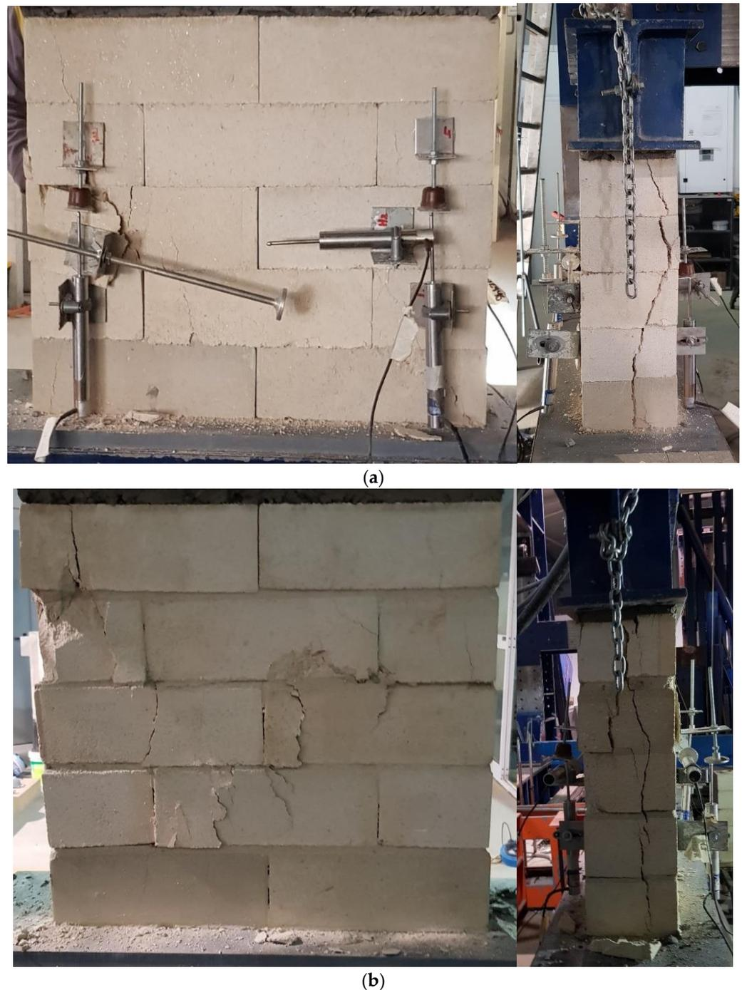
**Figure 11.** Failure mode of the wallets: (a) DSW and (b) MW.
