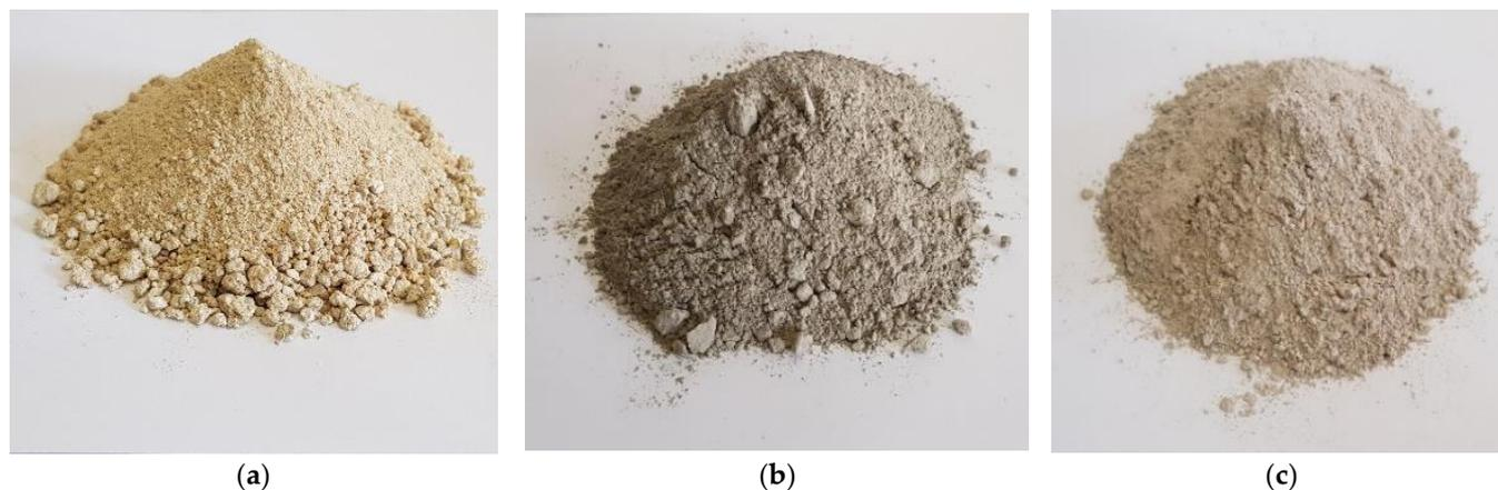
**Figure 2.** Raw materials used to produce the iCEBs: (a) soil; (b) cement; and (c) hydraulic lime.
