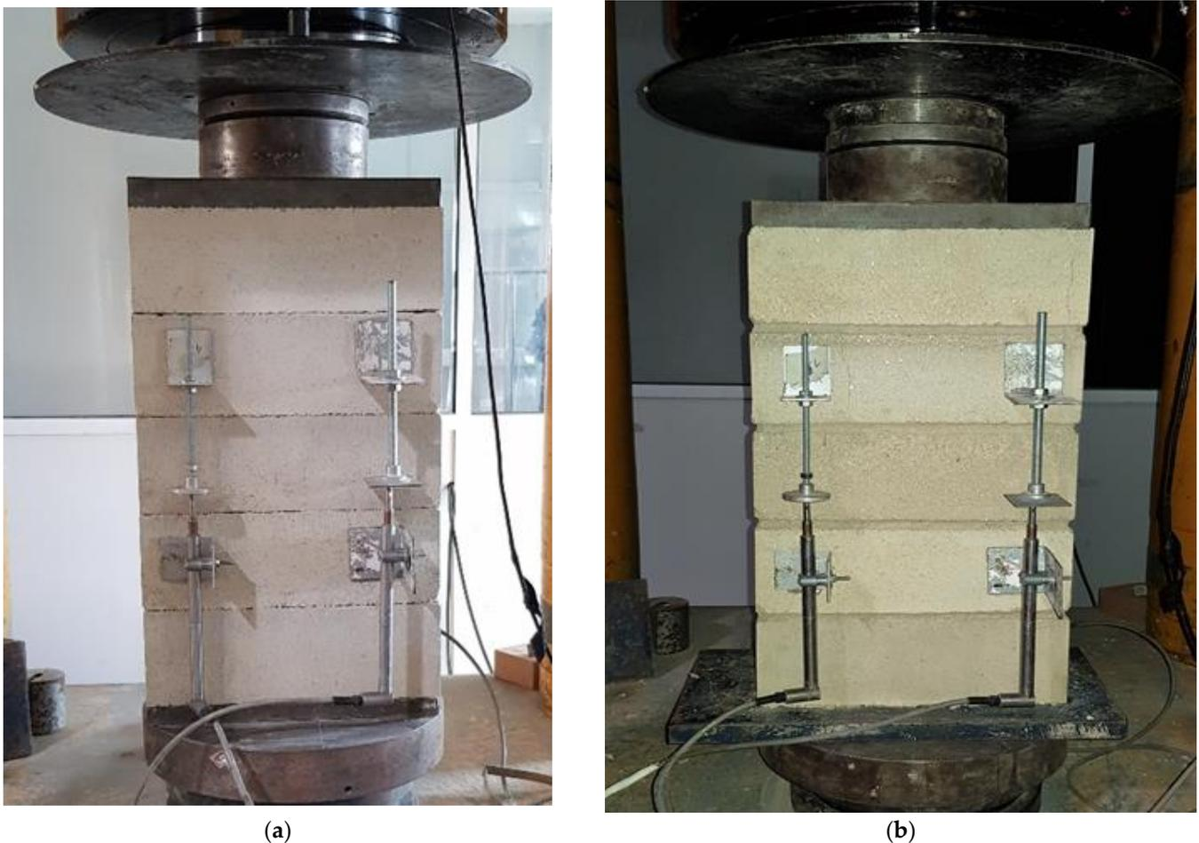
**Figure 6.** Setup of the compression tests conducted on masonry prisms: (a) DSP and (b) MP.
