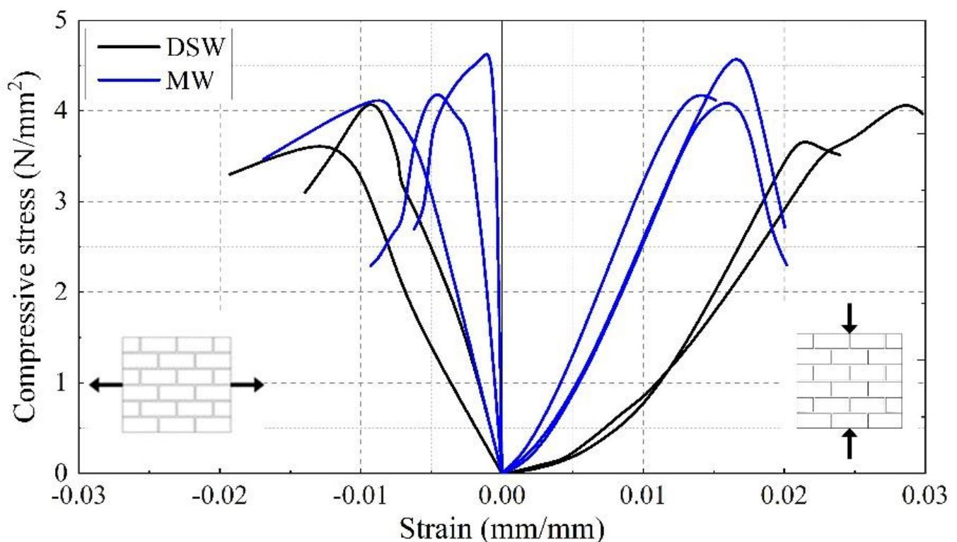
**Figure 10.** Stress–strain curves in compression of the wallettes with dry stack (DSW) and mortar joints (MW).
