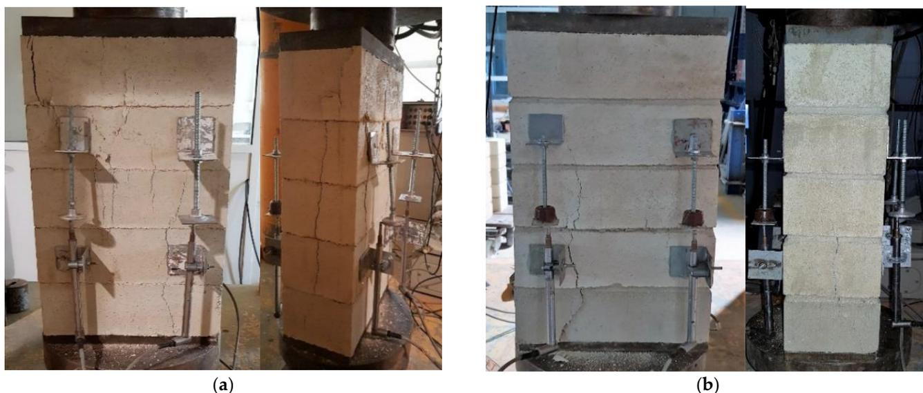
**Figure 9.** Failure mode of the prisms: (a) DSP and (b) MP.
