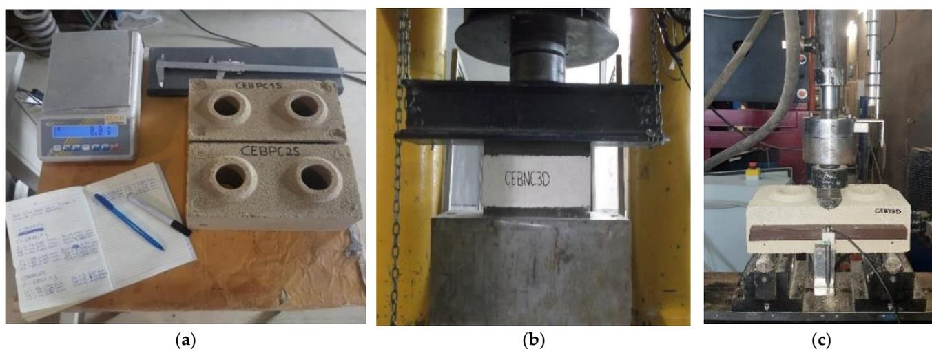
**Figure 5.** Test set-up for the characterization of the iCEBs produced: (a) geometrical stability; (b) compression test; and (c) three-point bending test.
