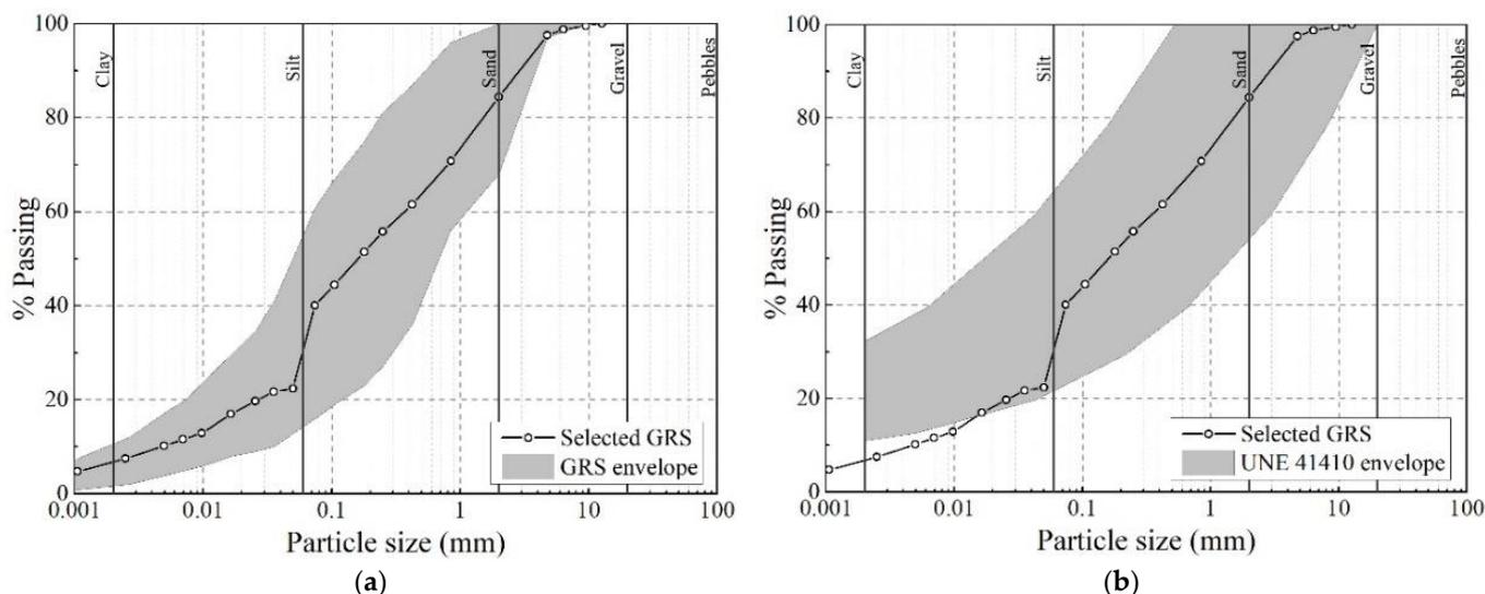
**Figure 3.** PSD of the selected soil and comparison with the envelope of (a) GRSs from Northern Portugal, according to Viana da Fonseca [37] and (b) soils recommended for CEBs production, according to UNE 41410 [39].
