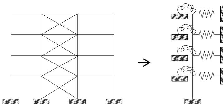
**Figure 5.** Model of a braced frame equivalent to a shear wall according to Carpinteri et al.
