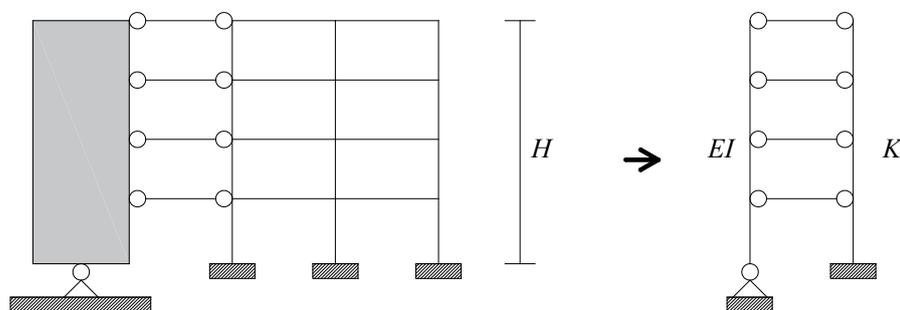
**Figure 7.** Equivalent model of frame hinged shear wall structures according to Bozdogan.
