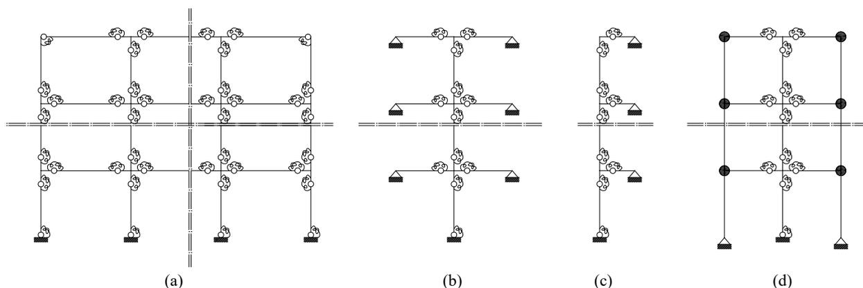
**Figure 10.** (a) Frame building (b) fishbone model (c) generic frame model (d) modified fishbone model.
