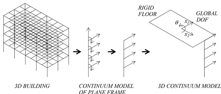
**Figure 3.** Construction of a 3D building model using continuum models for each plane frame according to McCallen and Romstad.
