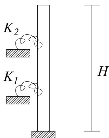
**Figure 2.** Schematization of the equivalent beam model proposed by Rahgozar et al.
