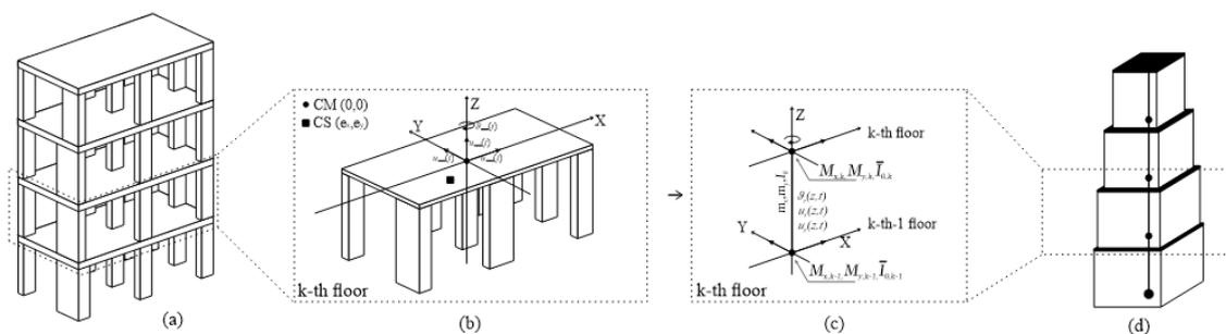
**Figure 6.** Concept of representation starting from (a) the 3D structure and (b) the generic k-th floor (or inter-storey) up to the (c) sub-beam element and the (d) proposed beam-like model. Source: own figure [58].
