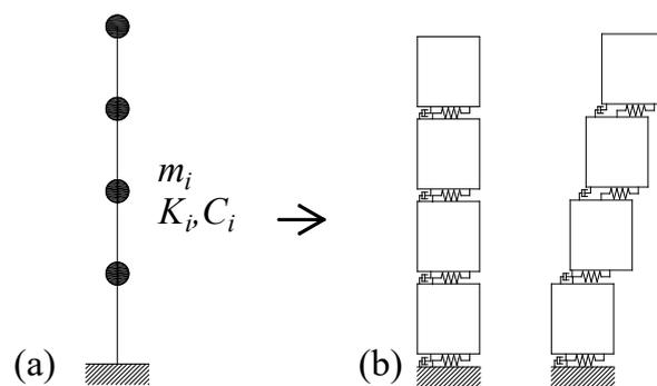
**Figure 9.** The multi-rigid-body model proposed by Lai et al. (a) shear-type model; (b) multi-rigid-body discrete model and displacements of the shear-type structure described by multi-rigid-body model.
