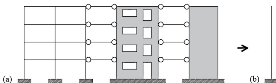
**Figure 4.** Model for lateral vibration analysis according to Zalka: (a) bracing system consisting of frames, coupled shear walls, shear walls and cores; (b) equivalent column.
