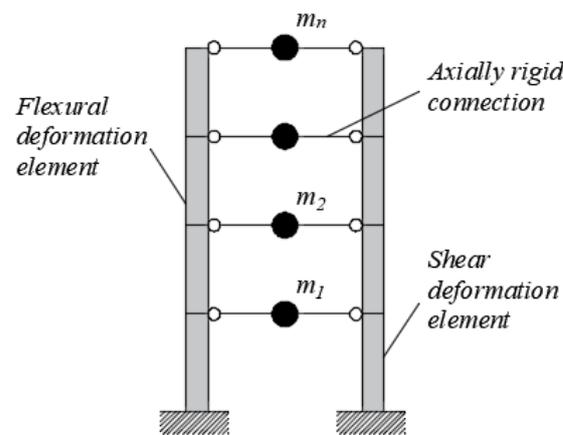
**Figure 11.** Mass distribution, flexural and shear deformation elements and floor links in the model proposed by Kuang and Huang.
