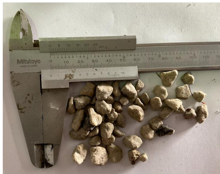
**Figure 1.** Lightweight aggregates.
