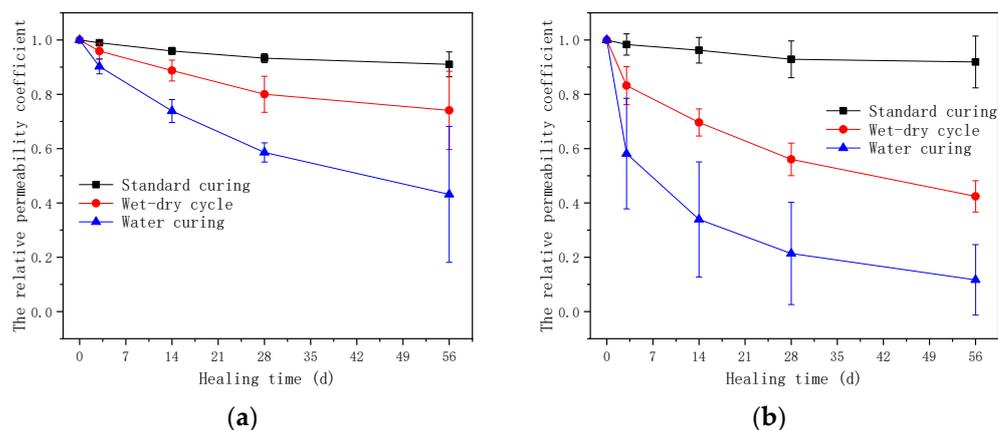
**Figure 5.** The relative permeability coefficient of mortar specimens under different exposure environments: (a) control; (b) with bacteria. Three specimens were tested for each exposure environment.
