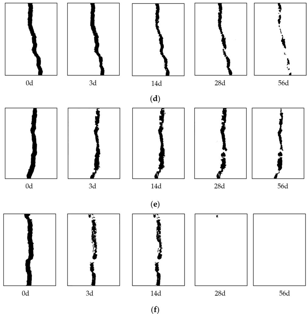
**Figure 3.** Binarized self-healing images of surface cracks in mortars under different exposure environments. (a) The control mortar specimens under the standard curing. (b) Mortar specimens with bacteria under the standard curing. (c) The control mortar specimens under the dry–wet cycle curing. (d) Mortar specimens with bacteria under the dry–wet cycle curing. (e) The control mortar specimens under the water curing. (f) Mortar specimens with bacteria under the water curing.
