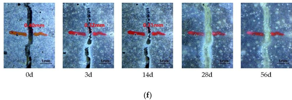
**Figure 2.** Self-healing images of surface crack in mortars under different exposure environments. (a) The control mortar specimens under the standard curing. (b) Mortar specimens with bacteria under the standard curing. (c) The control mortar specimens under the dry–wet cycle curing. (d) Mortar specimens with bacteria under the dry–wet cycle curing. (e) The control mortar specimens under the water curing. (f) Mortar specimens with bacteria under the water curing.
