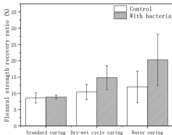
**Figure 6.** Flexural strength recovery ratio of mortar specimens under different exposure environments. Three specimens were tested for each exposure environment.
