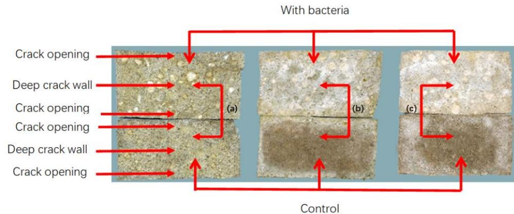
**Figure 7.** Healing products in crack wall of mortar specimens after healing for 56 d under different exposure environments: (a) standard curing; (b) dry–wet cycle; (c) water curing.
