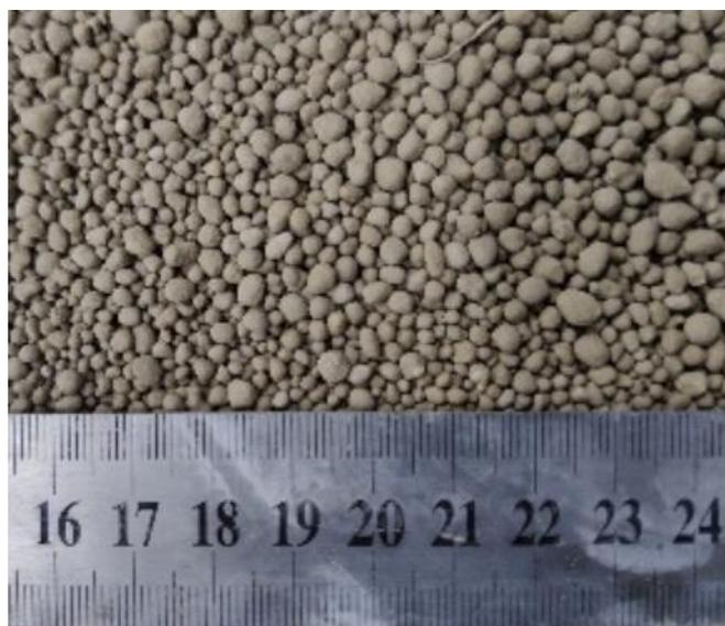
**Figure 1.** The artificial-functional-carrier-encapsulated bacteria.
