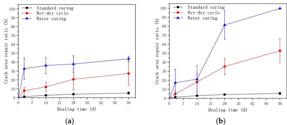
**Figure 4.** Crack area repair ratio of mortars under different exposure environments: (a) control; (b) with bacteria. Three specimens were tested for each exposure environment.
