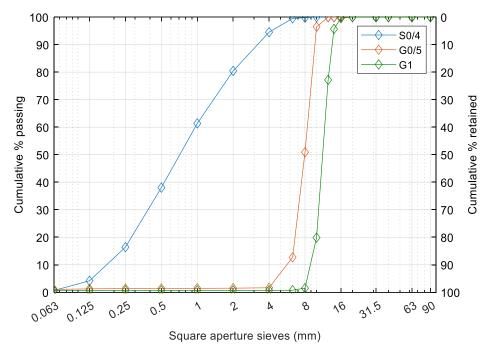
Figure 1. Particle size distribution of the mineral aggregates.
