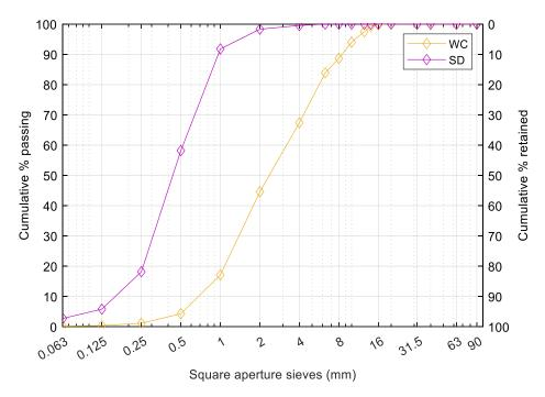
**Figure 3.** Particle size distribution of wood chips (WC) and sawdust (SD).
