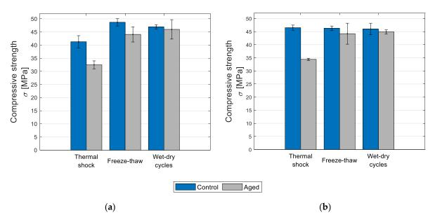
Figure 14. Artificial aging cycles: (a) WC25; (b) WC20SD5.
