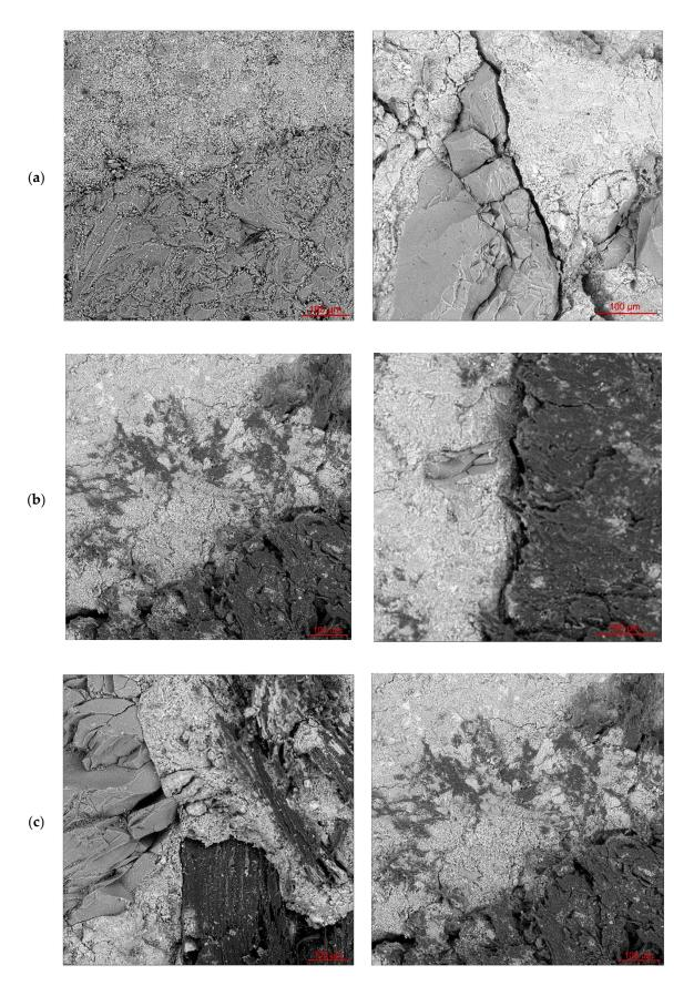
**Figure 8.** SEM micrographs with and without evidence of micro-cracking in the interface between aggregates and cement matrix in the right and left column, respectively: (a) REF; (b) WC25; (c) WC20S5.
