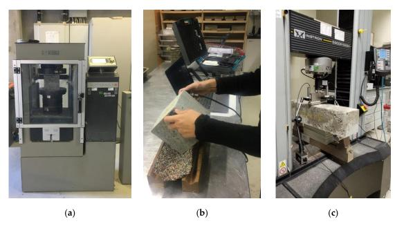
**Figure 4.** Mechanical characterization tests: (a) compressive strength; (b) dynamic modulus of elasticity; (c) flexural strength.
