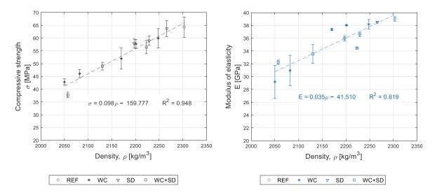
Figure 10. Variation in the compressive strength and modulus of elasticity with density.
