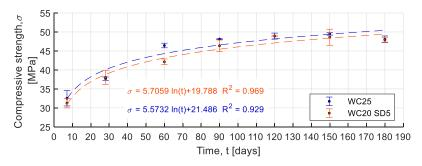
**Figure 13.** Compressive strength development over time (mean  $\pm$  standard deviation).
