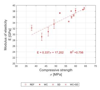
Figure 11. Variation of the modulus of elasticity with compressive strength.
