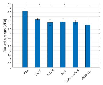
**Figure 12.** Flexural strength (mean values  $\pm$  standard deviation) for the wood–concrete samples at 28 days.
