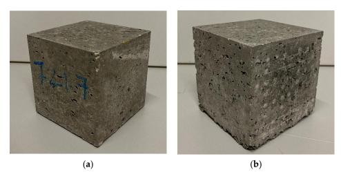
Figure 15. Test specimens after being subjected to wet-dry cycles: (a) WC25; (b) WC20S5.
