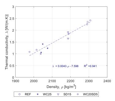
Figure 16. Relationship between thermal conductivity and density.
