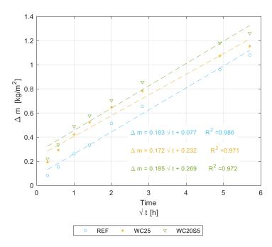
Figure 17. Mass gain per face area over time.
