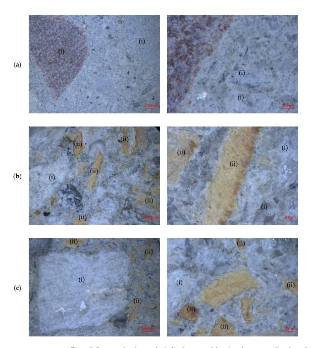
**Figure 7.** Stereoscopic micrographs, indicating some of the mineral aggregates (i) and wood particles (ii) embedded in the cement matrix: (a) REF; (b) WC25; (c) WC20S5.
