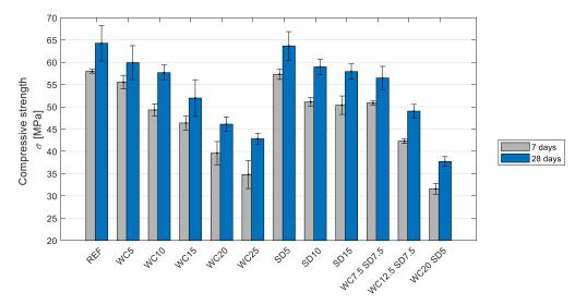
**Figure 5.** Compressive strength of the wood–concrete samples, mean values, and standard deviation at 7 days and 28 days.
