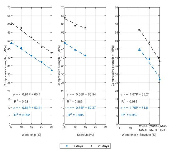
Figure 6. Mean values of compressive strength vs. wood percentage incorporated.
