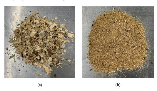
Figure 2. Wood aggregates: (a) wood chips (WC); (b) sawdust (SD).
