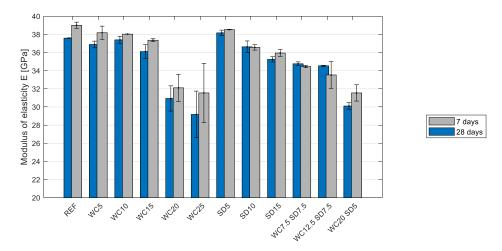
**Figure 9.** Modulus of elasticity of the wood–concrete samples (mean values  $\pm$  standard deviation) at 7 days and 28 days.
