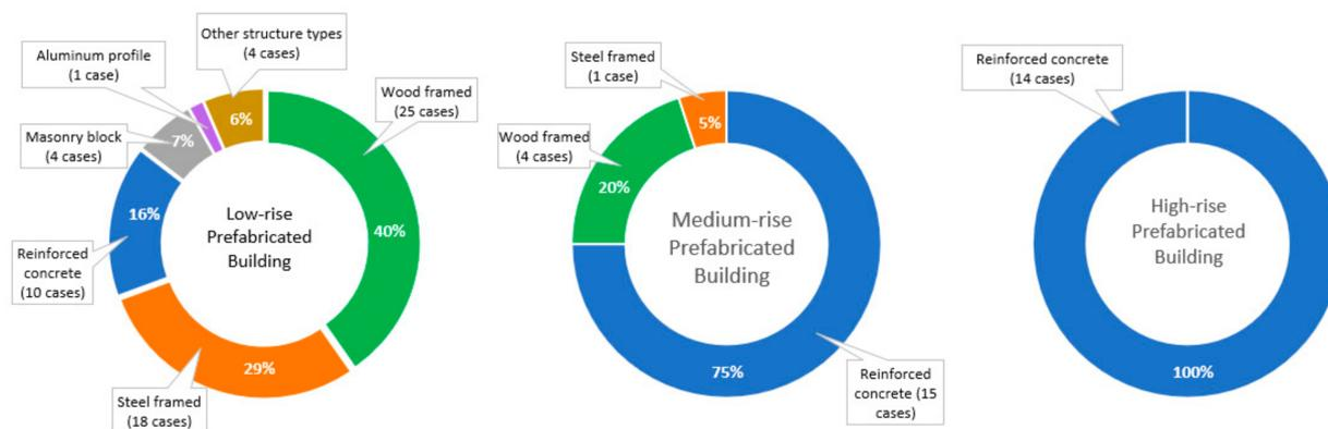
**Figure 10.** Relation between prefabricated building heights and building structural forms.
