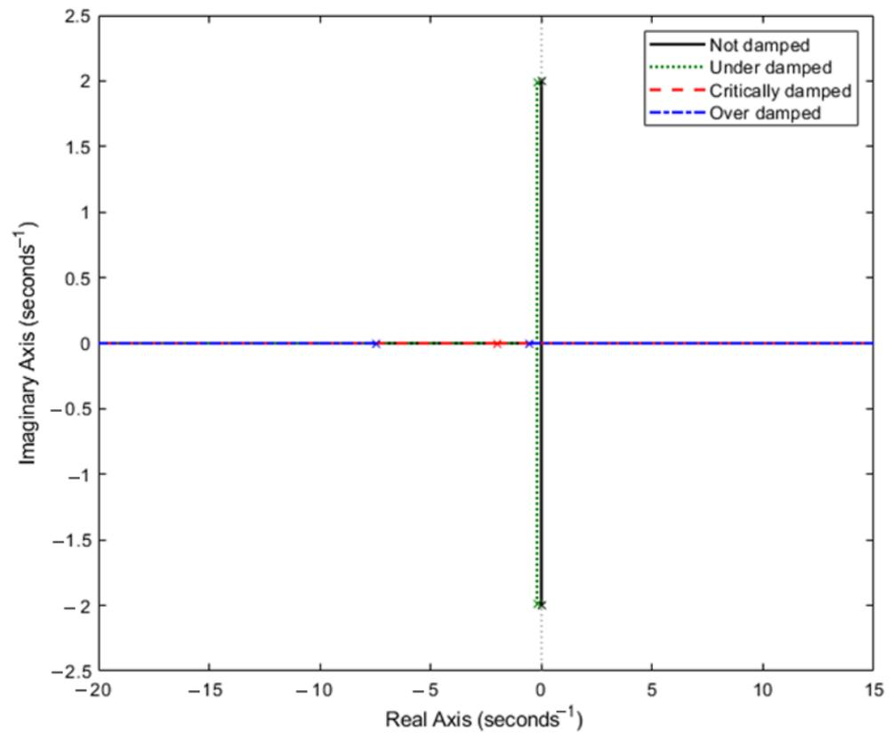
**Figure 7.** Root locus diagram of the lumped mass dynamic system (Case example 1) for four different arrangements of dominant eigenvalue/pole based on the system’s internal resistance/damping.
