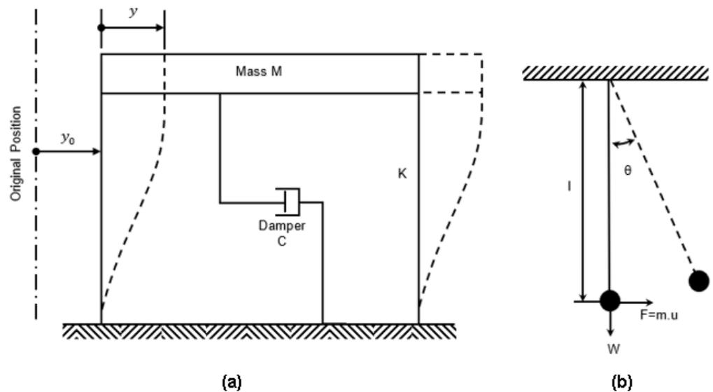
Figure 4. Two linear and nonlinear dynamic systems utilized in the study: (a) single degree of freedom structure subjected to a later loading. Source: adapted from Carmichael [21]. (b) A schematic diagram of a simple pendulum.
