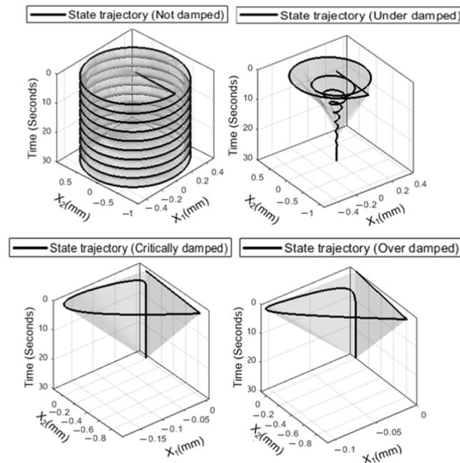
**Figure 13.** System phase portrait (domain of attraction) 3D representation as an indicator of engineering resilience. The vertical axis indicates settling time for a unit impulse input and  $[0, 0]$  initial conditions (Case example 1).
