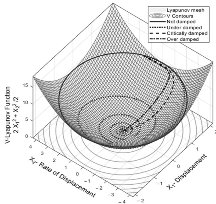
**Figure 8.** Lyapunov function (V), indicative of global asymptotic stability for the lumped mass dynamic system (Case example 1) along with the system phase portraits under [2, 1.5] state initial value.
