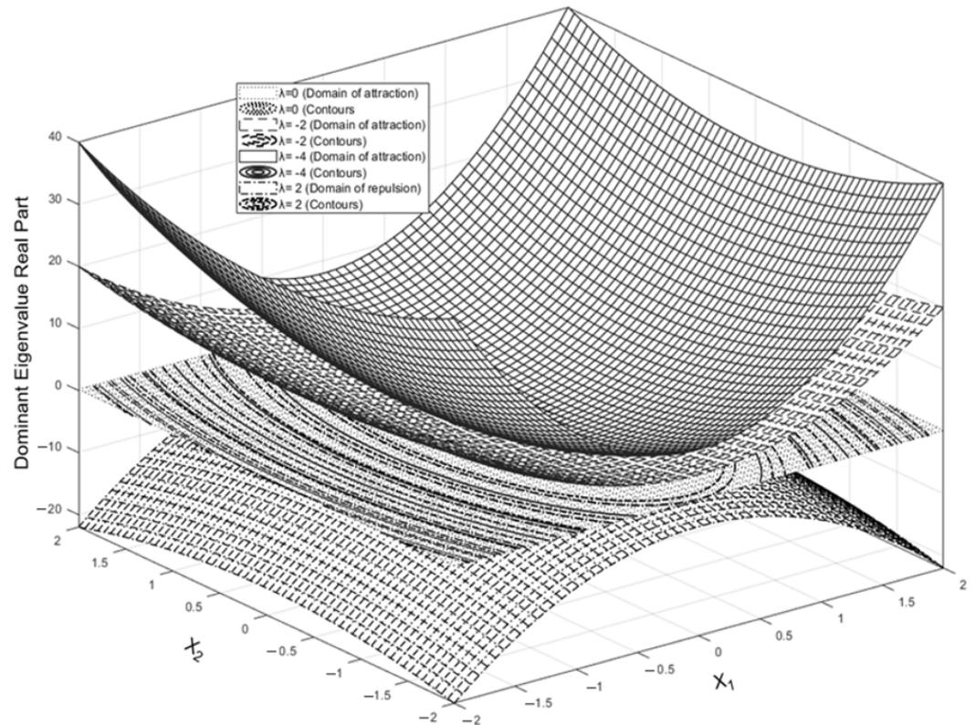
**Figure 15.** An approximate 3D representation of the equilibrium domain changes due to the system passive control levels. Dominant eigenvalue/pole real part indicate the rate of return to the equilibrium (Case example 1).
