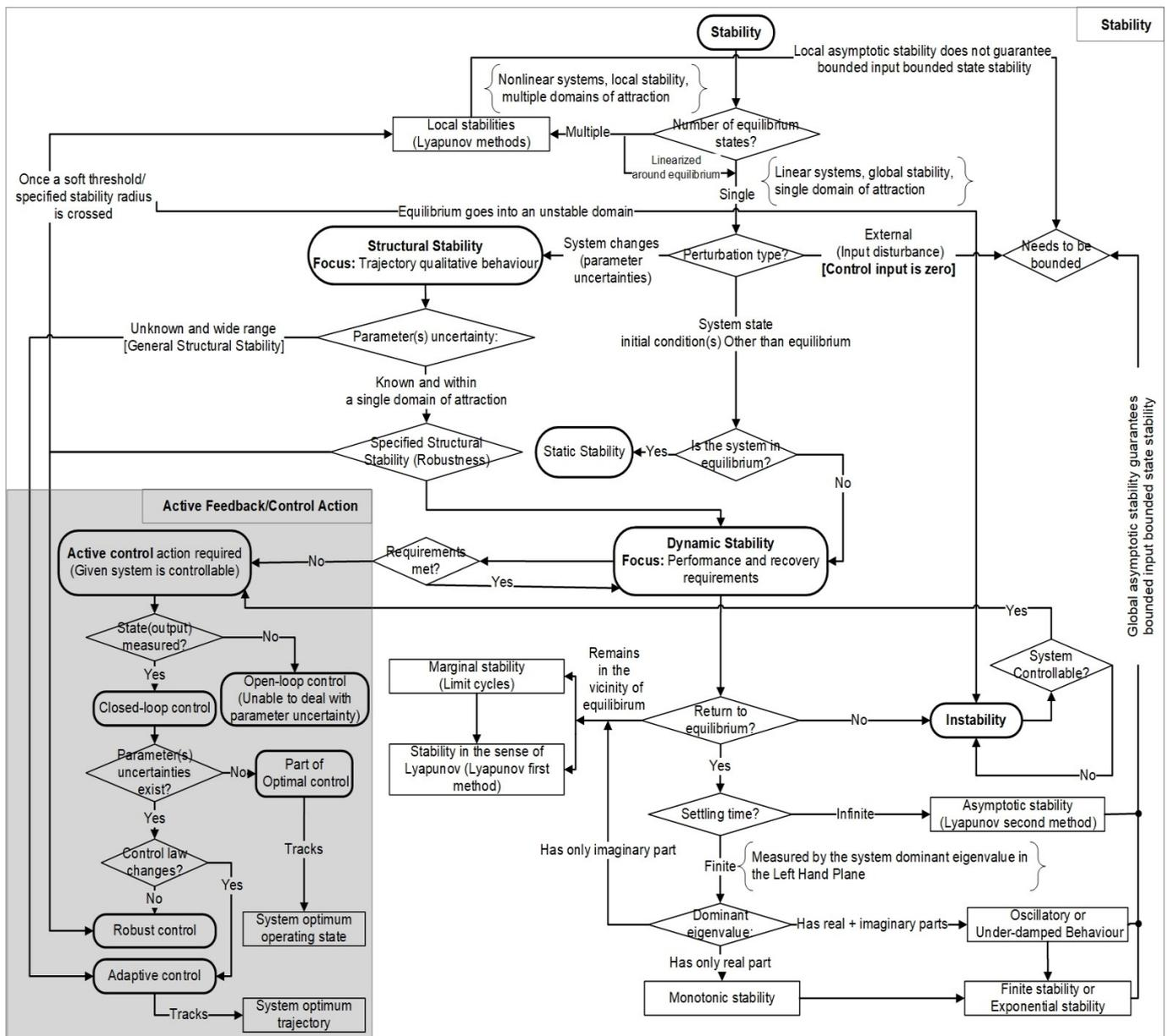
**Figure 6.** Linkages between dynamic stability, structural stability, and active control action—a unified and big picture.
