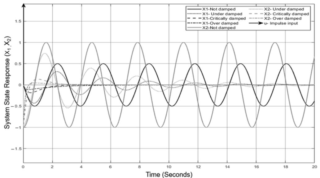
**Figure 12.** System state response under impulse input disturbance and  $[0, 0]$  initial conditions (Case example 1).
