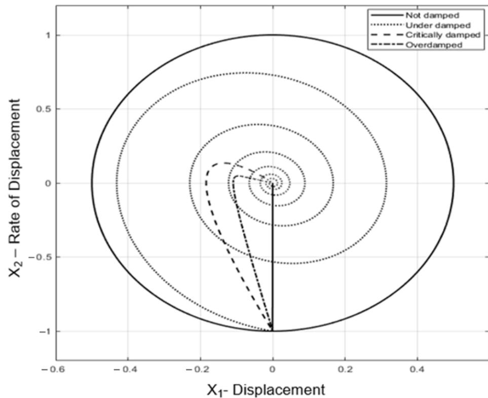
**Figure 11.** System phase portrait under unit impulse input disturbance and  $[0, 0]$  initial conditions (Case example 1).
