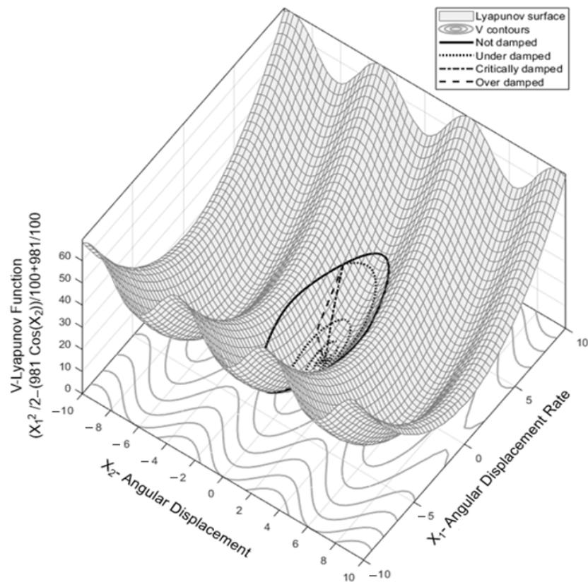
**Figure 9.** Lyapunov function (V) indicative of local asymptotic stability for the simple pendulum system (Case example 2) along with the system phase portraits under  $[-1.5 \text{ rad}, 4]$  state initial values.
