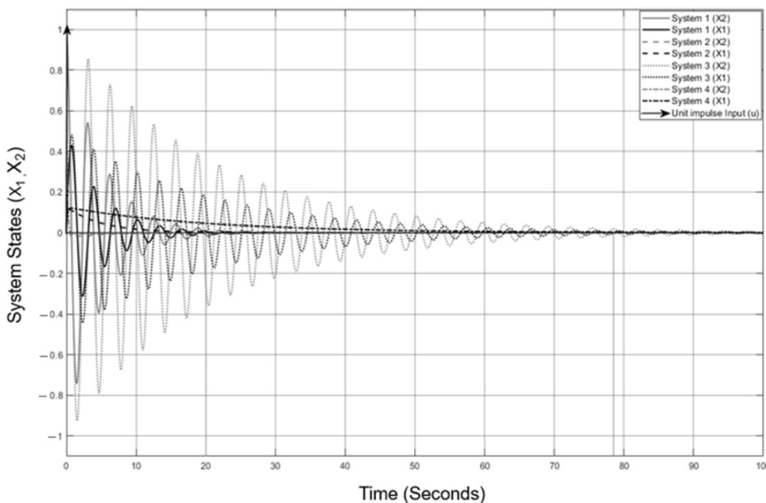
**Figure 10.** System equal dominant eigenvalues rendering equal settling times for a unit impulse in the form of a temporary input disturbance (Case example 1).
