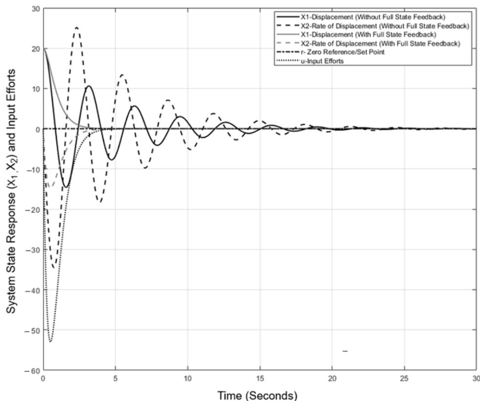
**Figure 20.** System state response with and without full state feedback (closed-loop control) for a zero reference/set point (equilibrium state) and  $[20\ 0]$  initial condition (Case example 1).
