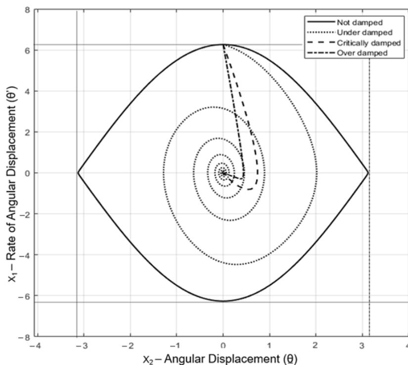
**Figure 16.** Phase portrait indicative of the system’s soft thresholds disturbed by initial conditions (Case example 2).
