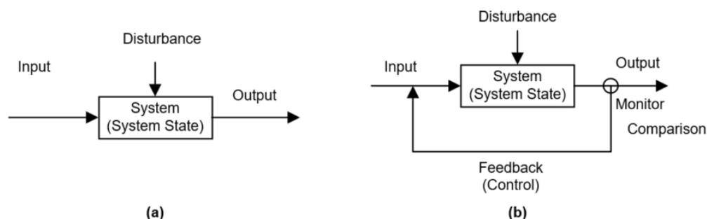
**Figure 5.** Flow of information for: (a) open-loop and (b) closed-loop representation of a dynamic system. Source: adapted from Carmichael [44].
