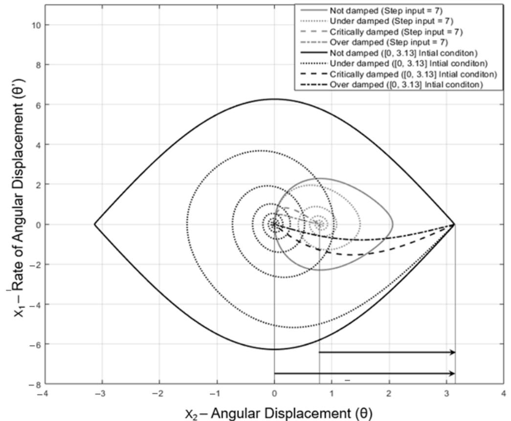
**Figure 17.** Permanent input (step input) acting as a parameter (input perturbation) that moves the system equilibrium state and affects resilience (Case example 2).
