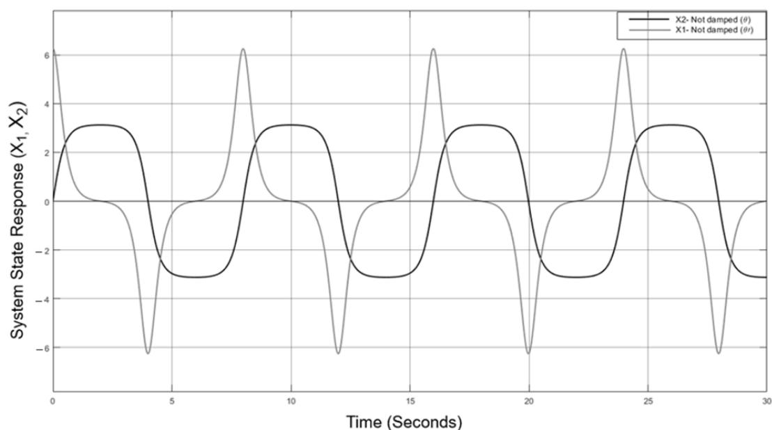
**Figure 14.** System state response indicative of the critical slowing down near an unstable equilibrium threshold (Case example 2 with  $[0, 6.264]$  initial conditions).
