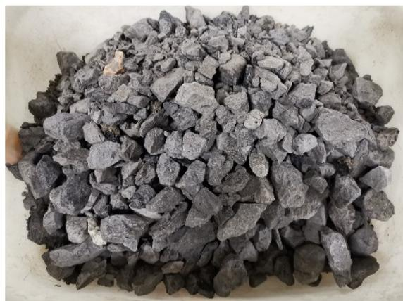
Figure 1. Coal gangue coarse aggregate (CGCA).
