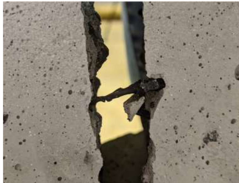
Figure 4. Crack bridging by tire shreds [23].
