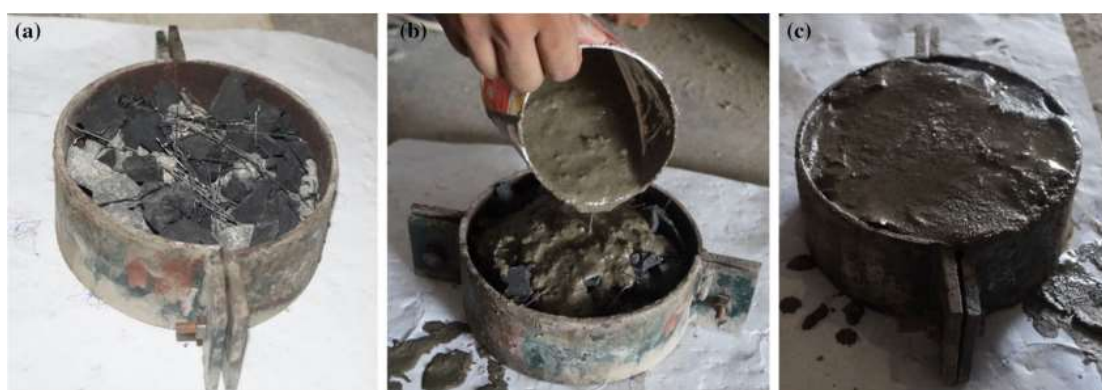
Figure 23. Preparation process of rubber concrete. (a) Arrange coarse aggregate, rubber and steel fibers. (b) Gravity method. (c) Sample [71].
