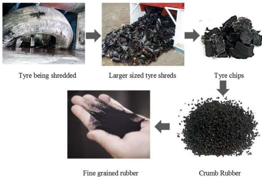
Figure 3. Different stages of tire shredding [22].
