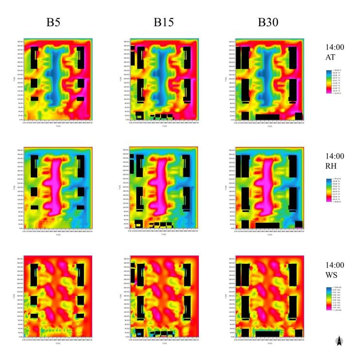
**Figure 9.** Distribution maps of microclimate parameters at 14:00 with redesigned building heights and densities.
