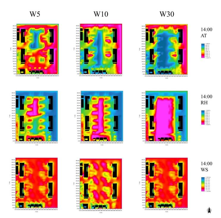
Figure 7. Distribution maps of microclimate parameters at 14:00 with redesigned water body coverage.
