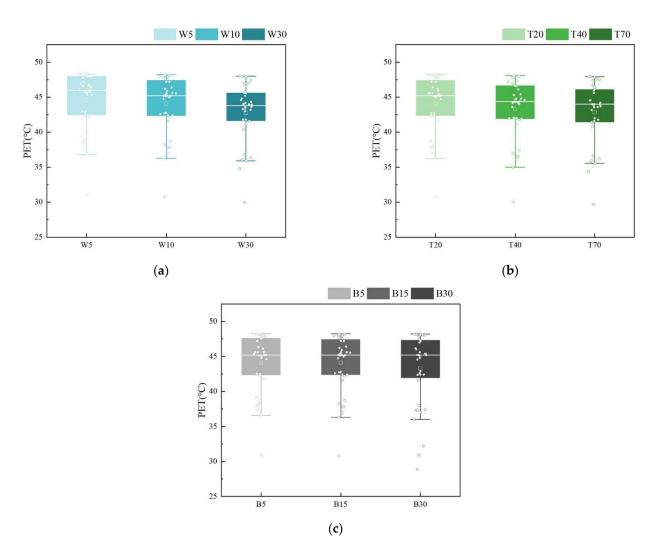
**Figure 12.** Box plots of PET from 9:00 to 18:00 vs. different quantities of (**a**) water bodies; (**b**) vegetation; and (**c**) buildings.
