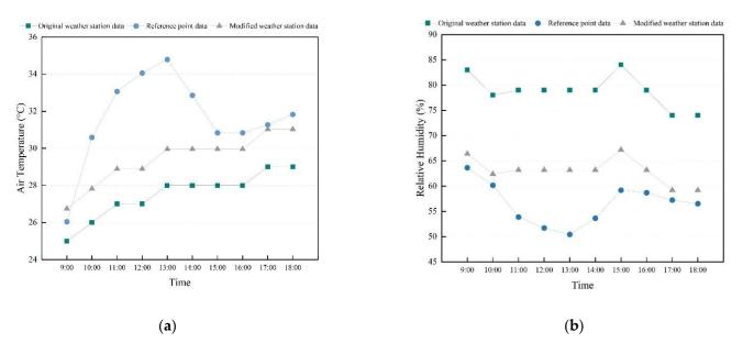
Figure 3. The comparison of the reference point data and weather station data: (a) AT; (b) Rh.
