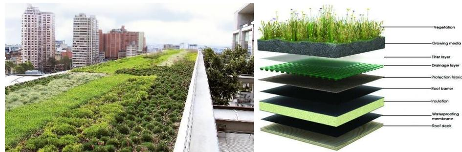
Figure 4. Green roof and its consisting layers.
