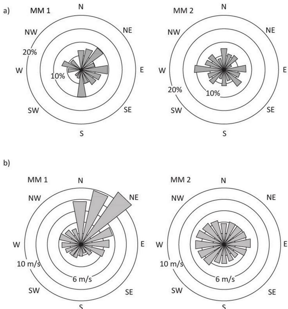
**Figure 7.** Distribution of (a) frequencies and (b) medium speed of wind direction at the observed meteorological stations for the periods 1998–2002 (for MM1) and 2000–2002 (for MM2) (adapted with permission from [43], Croatian Association of Civil Engineers, 2003).
