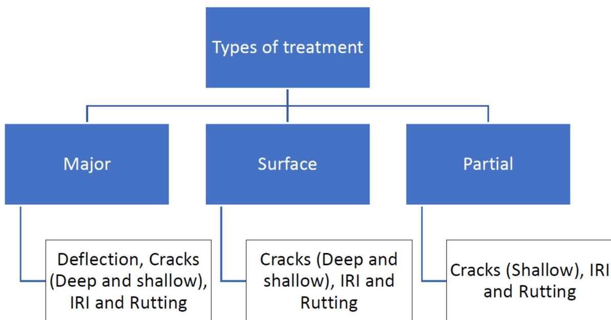
**Figure 5.** Types of maintenance treatment.
