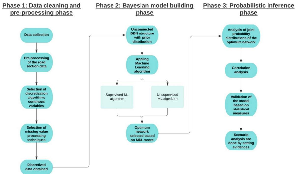
**Figure 6.** The framework of the proposed BBN model.
