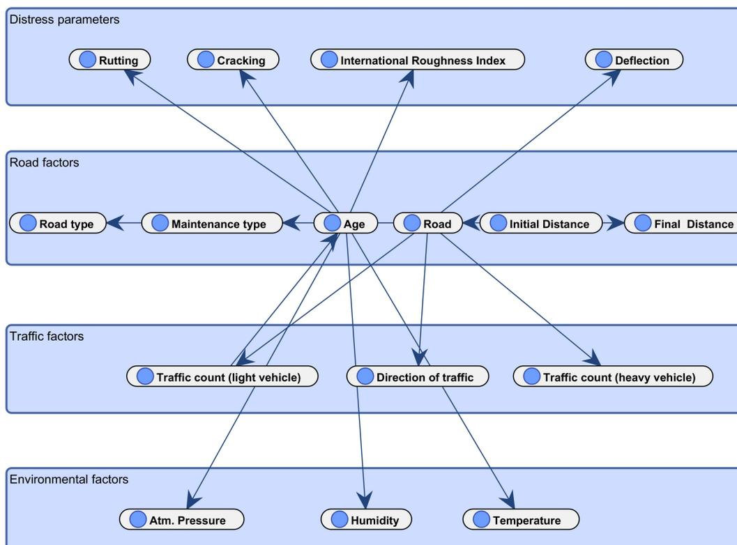
**Figure 9.** Bayesian network for road distress parameters, road factors, traffic factors and environmental factors.
