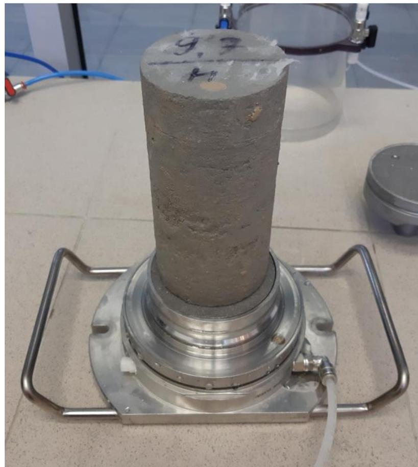
**Figure 1.** A fully water-saturated soil-cement specimen on the dismountable lower pedestal of the resonance column.
