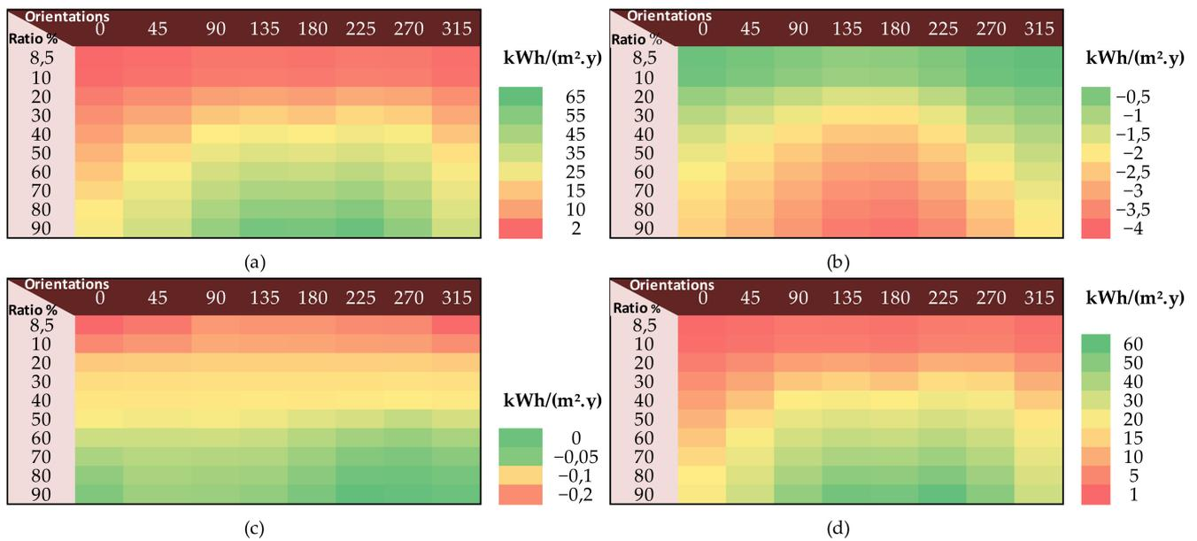
**Figure 6.** Variation in energy demand resulting from use of EC glazing instead of double glazing window, as a function of WWR and orientations for (a) cooling. (b) Heating. (c) Lighting. (d) Overall consumption. per unit area kWh/(m<sup>2</sup>.y).
