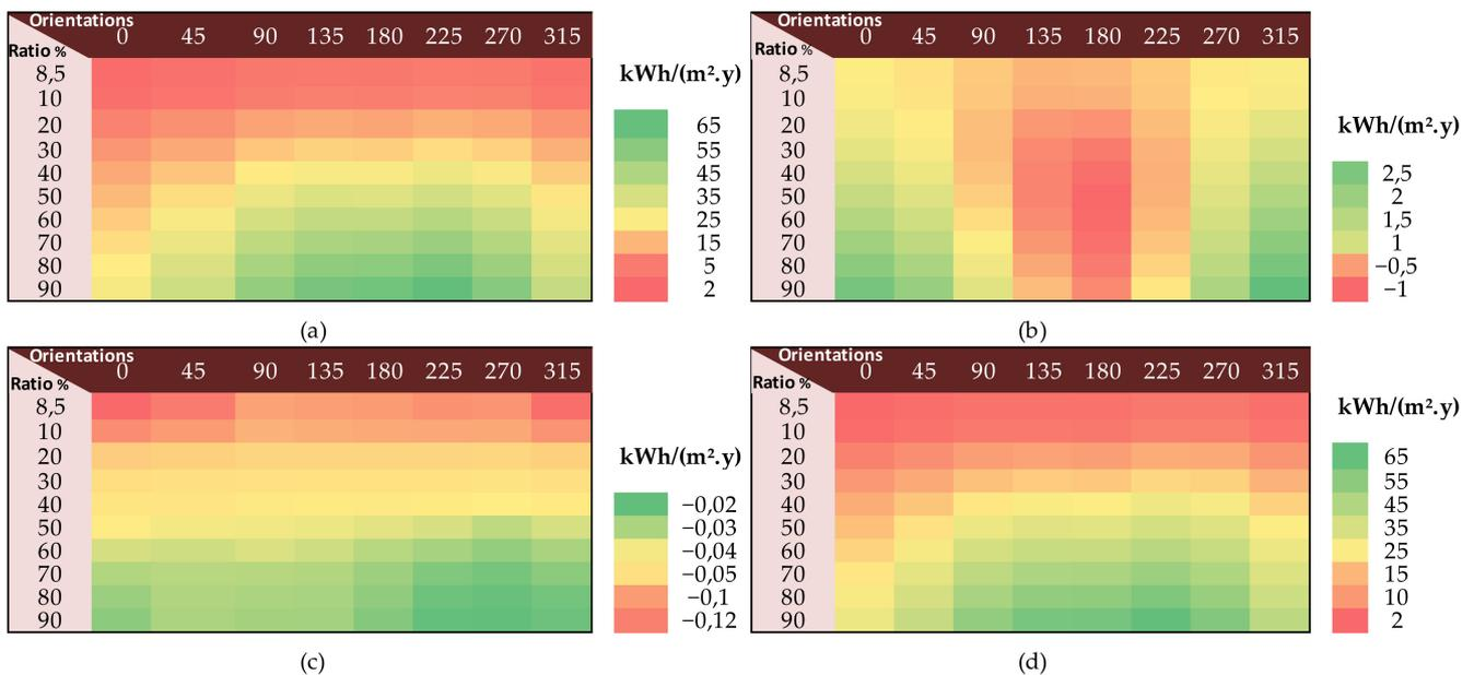
**Figure 7.** Variation in energy demand resulting from use of EC glazing instead of reference window, as a function of WWR and orientations for (a) Cooling. (b) Heating. (c) Lighting. (d) Overall energy consumption per unit area kWh/(m<sup>2</sup>.y).
