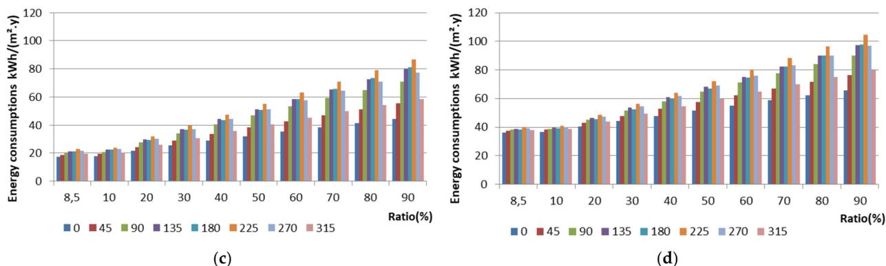
**Figure 5.** Electric energy consumptions for laminated glazing as a function of different orientations and WWR kWh/(m<sup>2</sup>.y). (a) Heating. (b) Lighting. (c) Cooling. (d) Overall consumptions.
