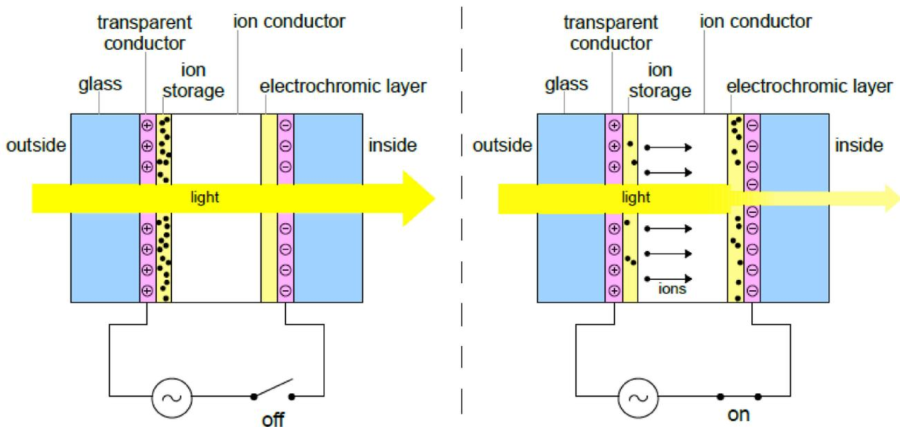
**Figure 1.** Electrochromic glazing schematic diagram.
