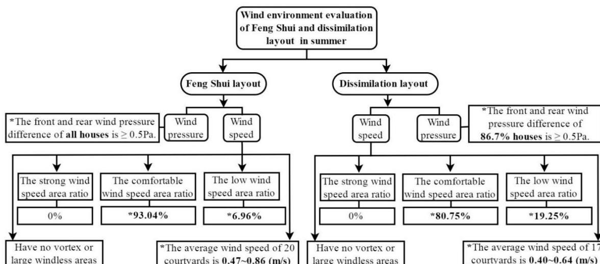
**Figure 14.** Outdoor wind environment evaluation of the feng shui layout and the dissimulation layout in summer (items with \* mean that there is a big difference between the two layouts).
