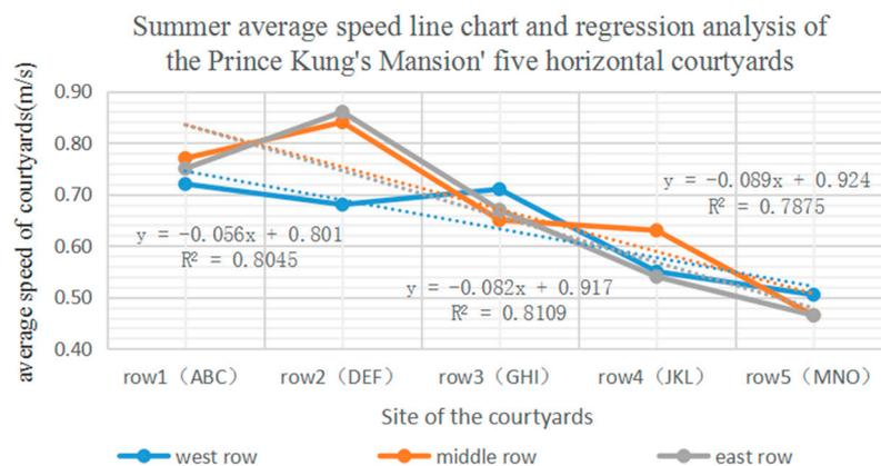
**Figure 12.** Average speed line chart and regression analysis of Prince Kung's Mansion' five horizontal courtyards in summer. The values of the figure was based on CFD simulation results.
