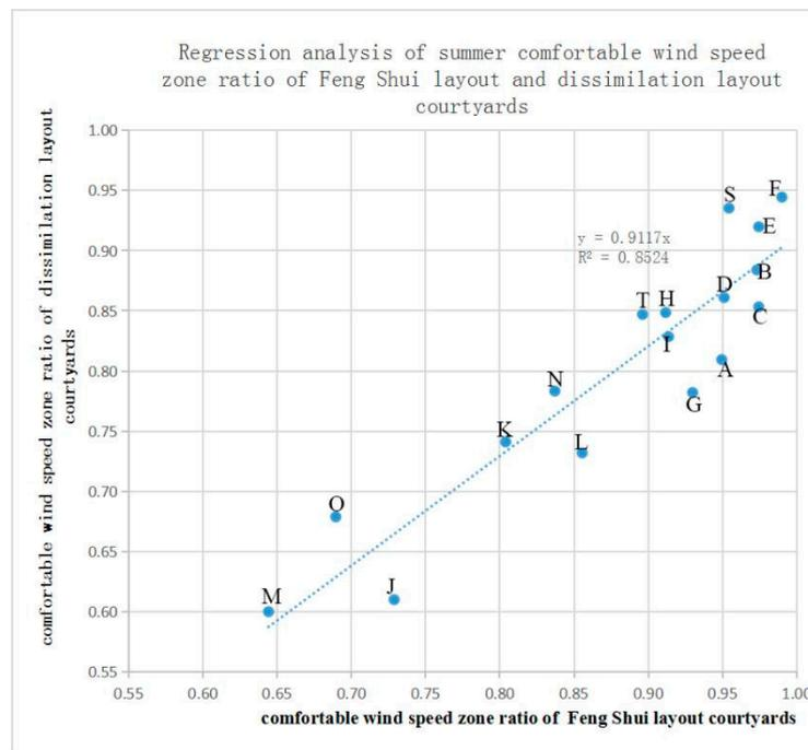
**Figure 11.** The regression analysis of the comfortable wind speed zone ratio for the courtyards of feng shui layout and dissimulation layout in summer. The values of the figure was based on CFD simulation results.
