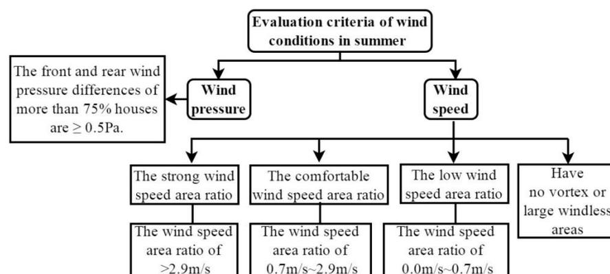
**Figure 3.** Diagram of the evaluation criteria for the outdoor wind environment.
