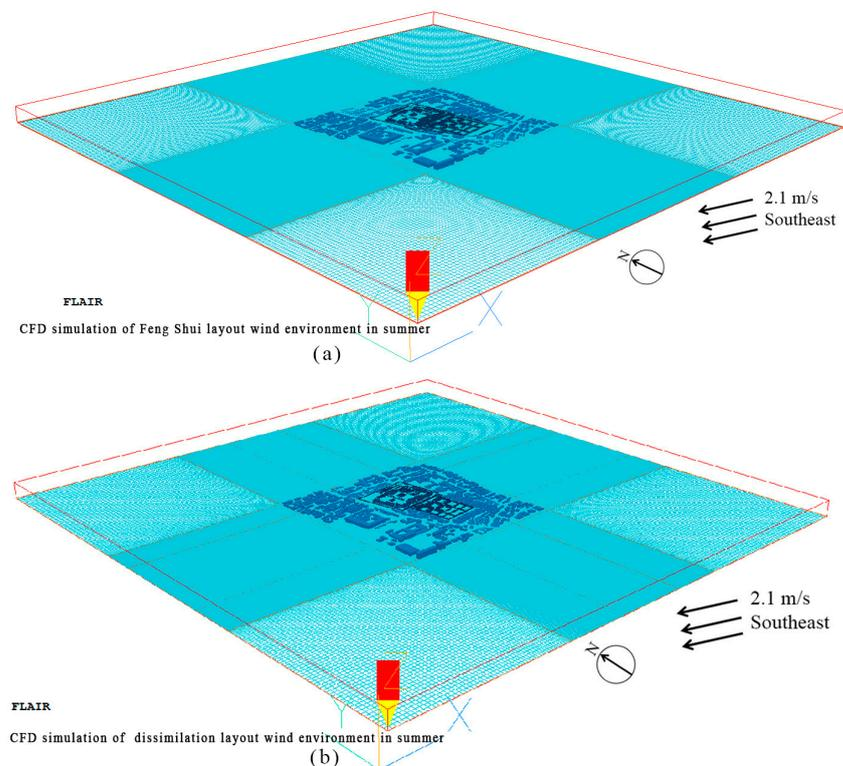
**Figure 4.** PHOENICS mesh settings: (a) the feng shui layout; (b) the dissimulation layout.
