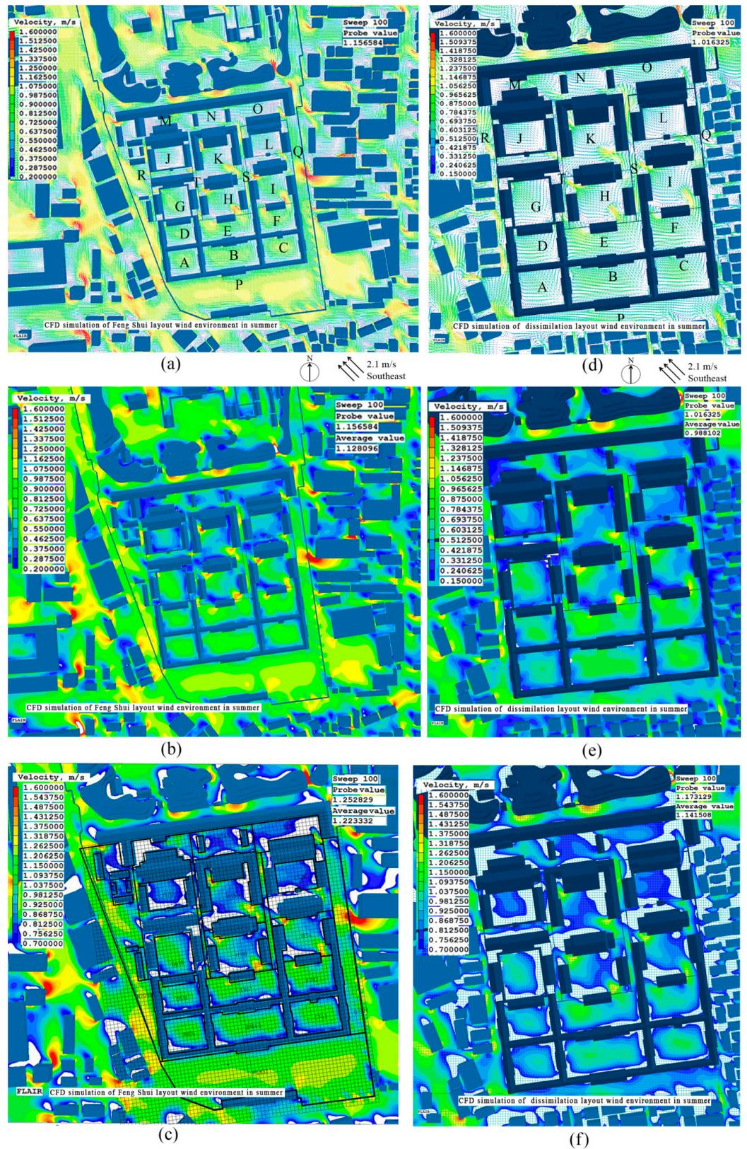
**Figure 7.** (a) Wind speed vector chart of feng shui layout. (b) Wind speed cloud chart of feng shui layout. (c) Comfortable wind speed zone cloud chart of feng shui layout. (d) Wind speed vector chart of dissimilation layout. (e) Wind speed cloud chart of dissimilation layout. (f) Comfortable wind speed zone cloud chart of dissimilation layout. The figures were obtained by CFD simulation.
