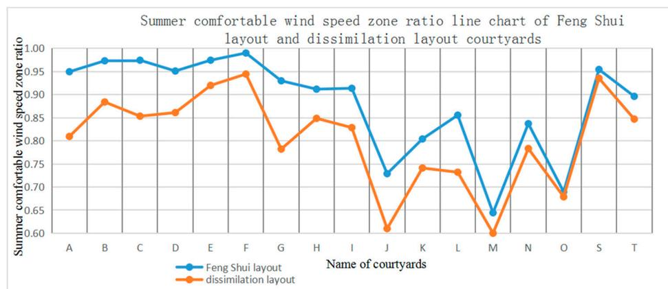
**Figure 10.** The comfortable wind speed zone ratio line chart for the courtyards of feng shui layout and dissimulation layout in summer. The values of the figure was based on CFD simulation results.
