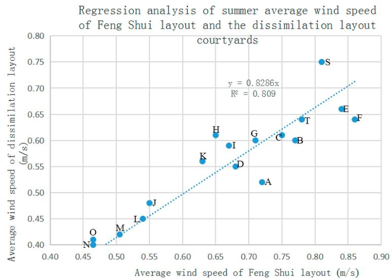
**Figure 9.** The regression analysis of the summer average wind speed for the courtyards of feng shui layout and dissimulation layout. The values of the figure was based on CFD simulation results.
