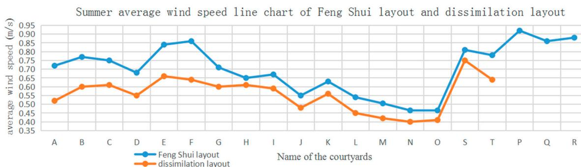
**Figure 8.** The average wind speed line chart for the courtyards of feng shui layout and dissimulation layout. The values of the figure was based on CFD simulation results.
