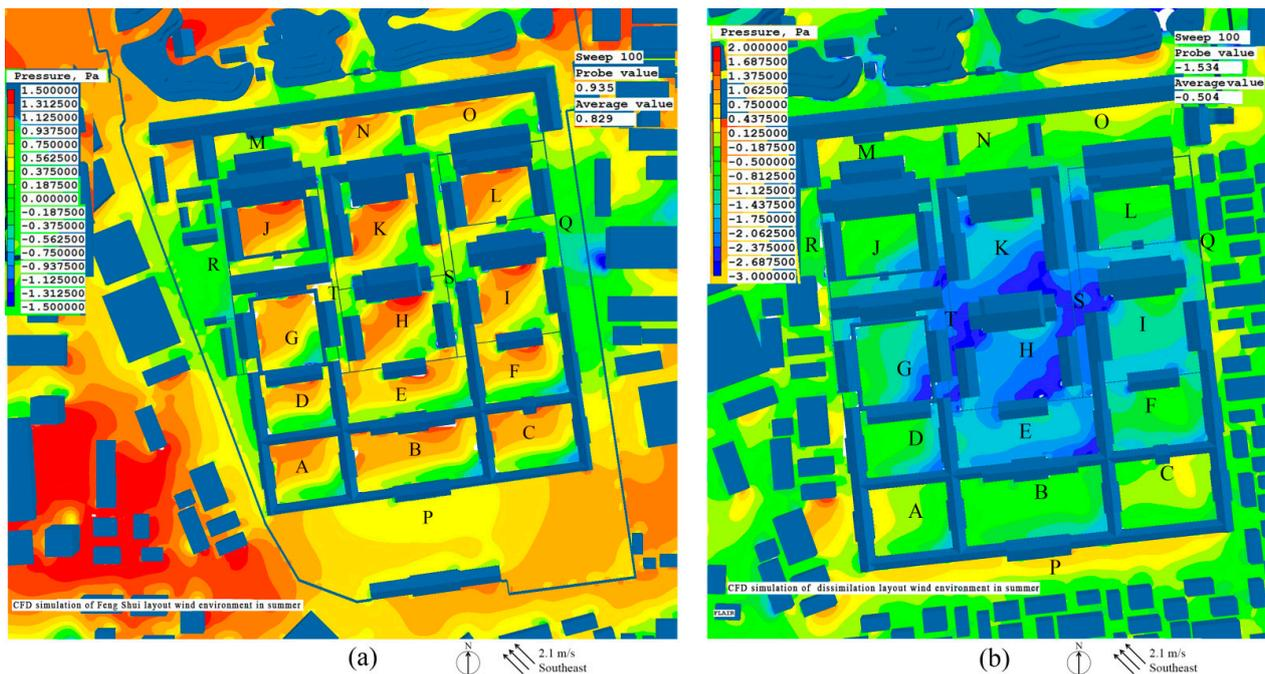
**Figure 13.** (a) Wind pressure cloud of feng shui layout in summer. (b) Wind pressure cloud of dissimilation layout in summer. The figures were obtained by CFD simulation.
