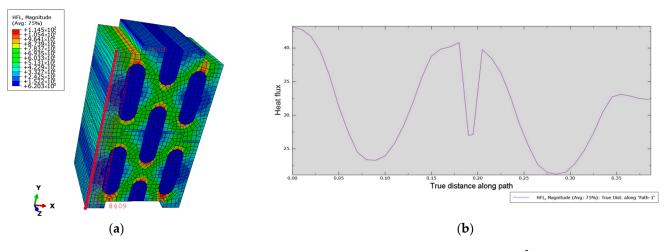
**Figure 3.** (a) Left calculation path in the 3D model; (b) heat flux  $(W \cdot m^{-2})$  of each node in the left path.
