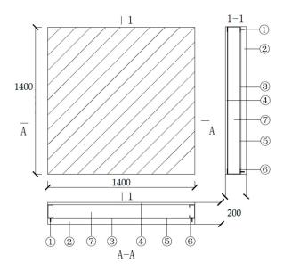
**Figure 1.** Configuration of LAEWP (unit: mm). ① steel stud, ② high strength concrete, ③ U-shape light-gauge steel, ④ fiber concrete board, ⑤ air layer, ⑥ C-shape light-gauge steel, and ⑦ EPS insulation layer.
