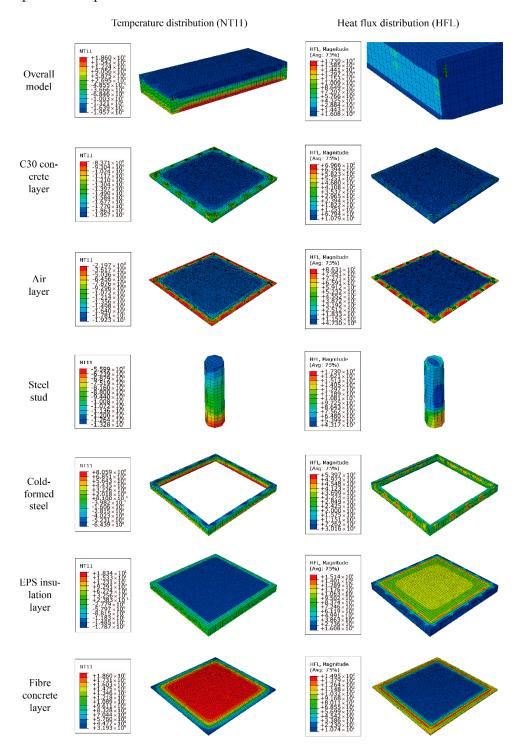
**Figure 6.** Temperature (°C) and heat flux  $(W \cdot m^{-2})$  distribution of NT11 and HFL of the LAEWP and all parts.
