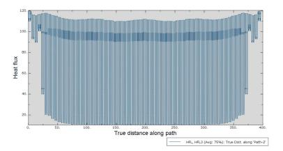
**Figure 8.** Heat flux  $(W \cdot m^{-2})$  of each node of fiber concrete.
