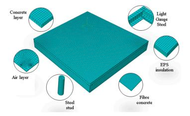
Figure 5. Mesh of the LAEWP and each component.
