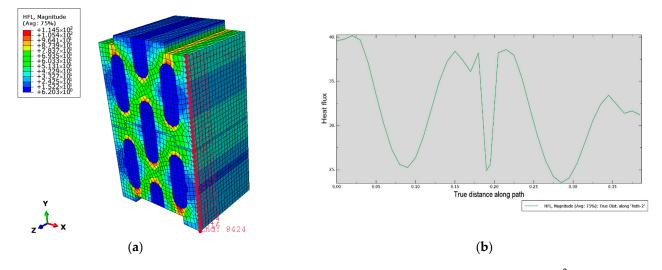
**Figure 4.** (a) Right calculation path in the 3D model; (b) heat flux  $(W \cdot m^{-2})$  of each node in the right path.
