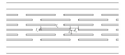
Figure 9. The layout of web openings of C light-gauge steel.
