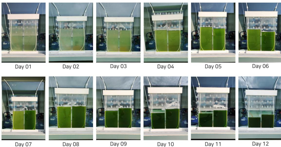
Figure 5. Change of microalgae's density during mock-up test (Adapted from Ref. [26]).
