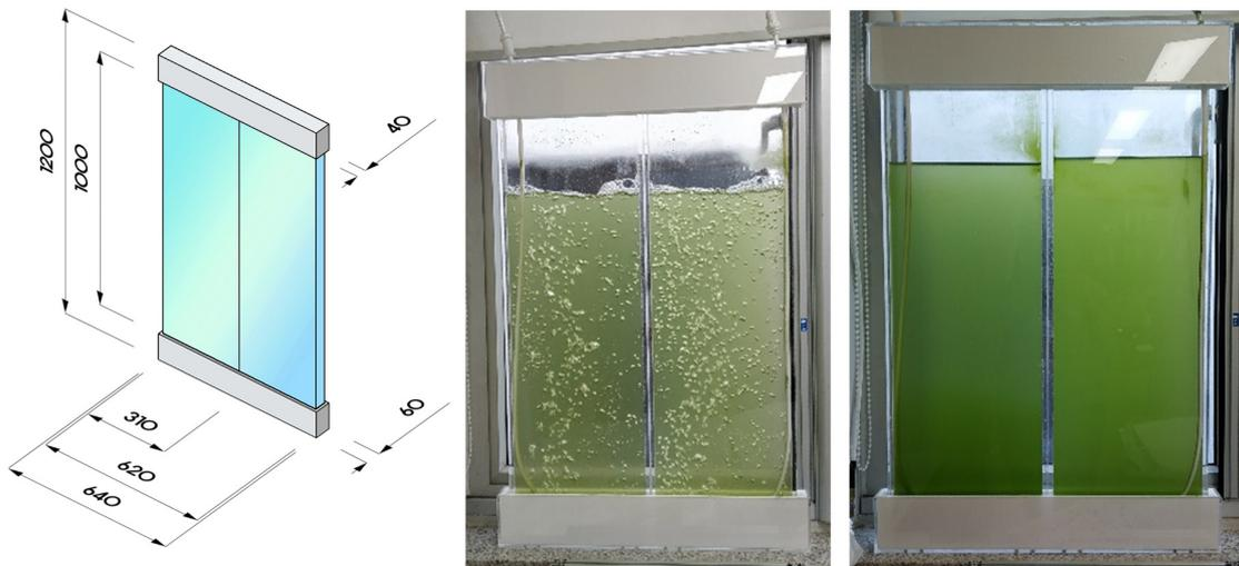
Figure 3. Test specimen of microalgae façade (Adapted from Ref. [26]).
