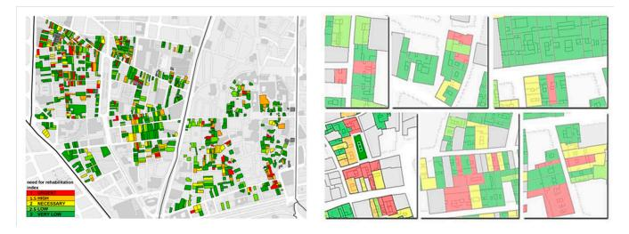
**Figure 2.** Examples of the disperse distribution of buildings in a poor state of conservation in the El Raval neighborhood (Adapted from Ref. [29]).
