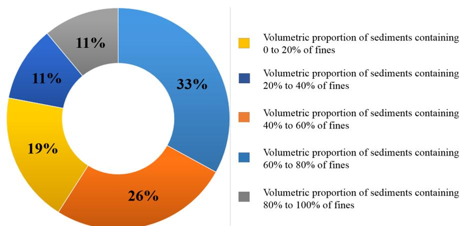
**Figure 1.** Volume proportion of dredged sediments according to their fines content (<50 µm).
