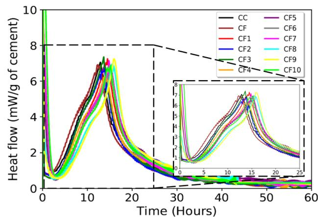
**Figure 4.** Heat flow–semiadiabatic calorimetry tests for different sediment-based concretes.
