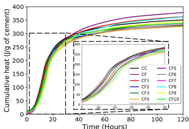
**Figure 3.** Cumulative heat–semiadiabatic calorimetry tests for different sediment-based concretes.
