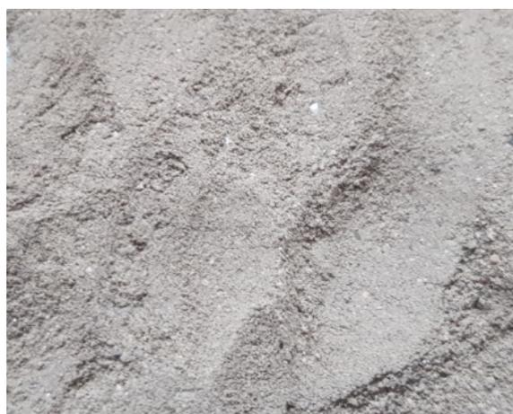
**Figure 2.** Fine sediments dried at 105 °C and crushed (<80 μm).
