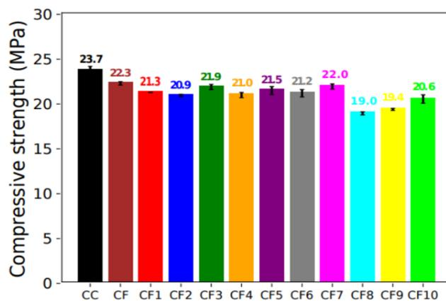
**Figure 5.** Compressive strength at 3 days.
