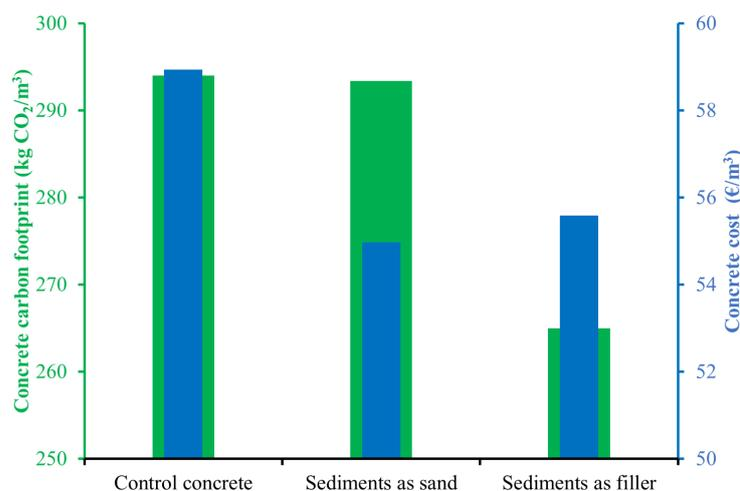
**Figure 9.** Carbon footprint and cost for different concretes (the green bars correspond to the carbon footprint and the blue bars correspond to the concrete cost).
