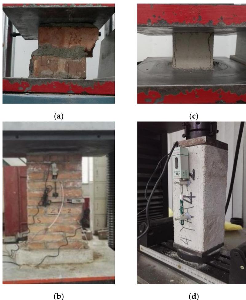
**Figure 2.** The testing of mechanical properties of brick (a), masonry (b) and mortar (c,d).
