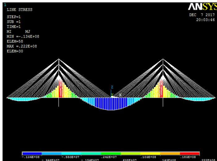
Figure 5. Bending moment distribution of main girder of cable-stayed bridge under dead load.
