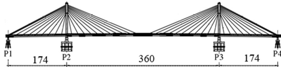
**Figure 3.** Structural size of the bridge.
