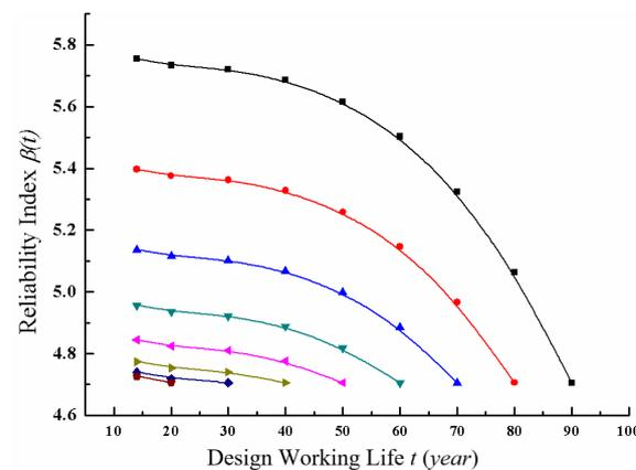
**Figure 10.** Time-varying reliability index of main girder of cable-stayed bridge with different initial reliability.
