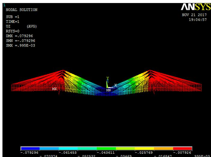
Figure 6. Deformation of main girder of cable-stayed bridge under vehicle load.
