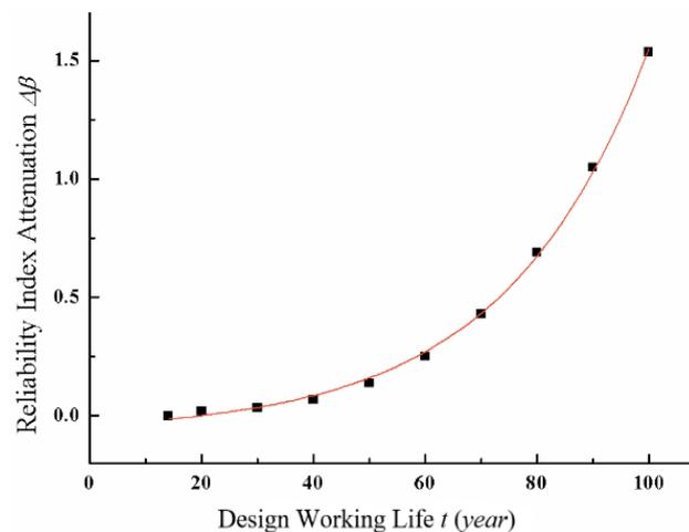
**Figure 9.** Reliability index degradation of main girder of cable-stayed bridge.
