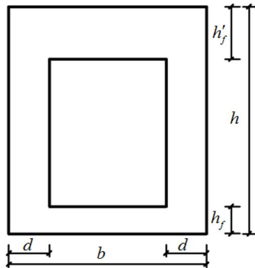
**Figure 2.** Box section model.
