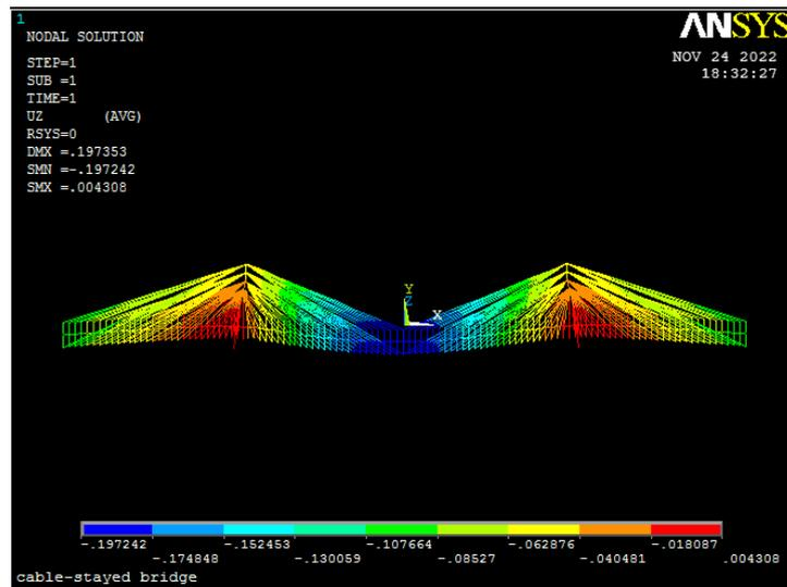
Figure 4. Deformation of main girder of cable-stayed bridge under dead load.
