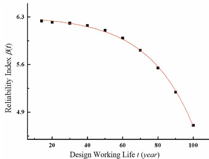
**Figure 8.** Time-varying reliability index of main girder of cable-stayed bridge.
