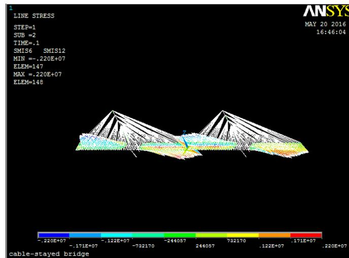
**Figure 7.** Bending moment distribution of main girder of cable-stayed bridge under vehicle load.
