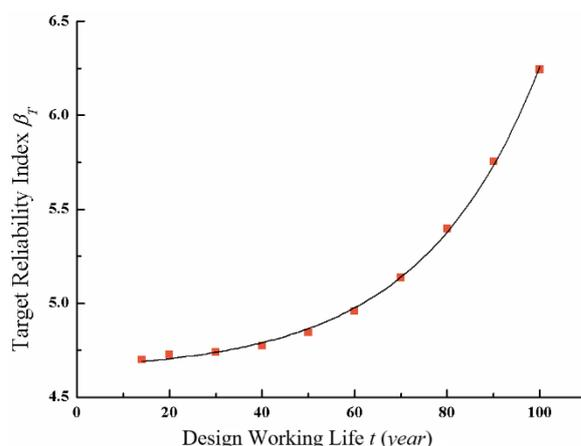
**Figure 11.** Relationship between target reliability index and design working life.
