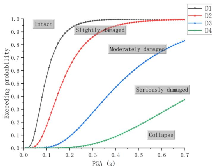
**Figure 5.** Probability of exceeding each failure state of prefabricated building structures at different PGA levels.
