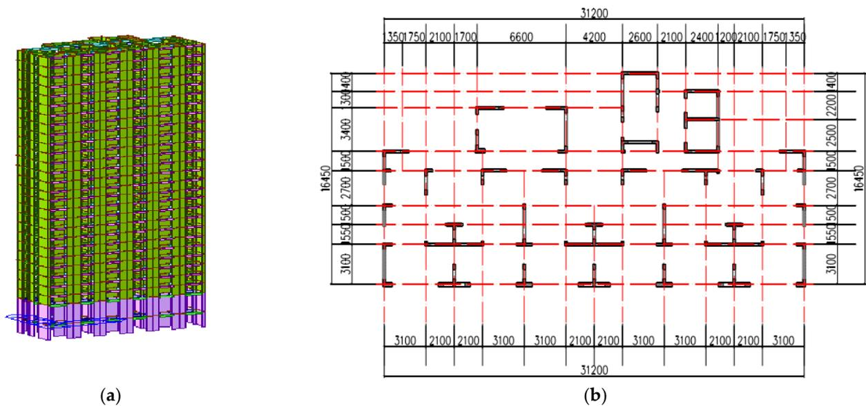
Figure 3. (a) Model of assembled shear wall structure; (b) Wall and column arrangement of the structure.
