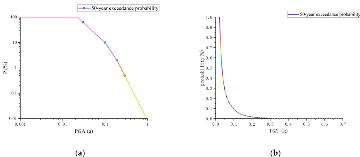
**Figure 6.** (a) Seismic hazard curve of the zone (logarithmic coordinates); (b) Seismic hazard curve of the zone (general coordinates).
