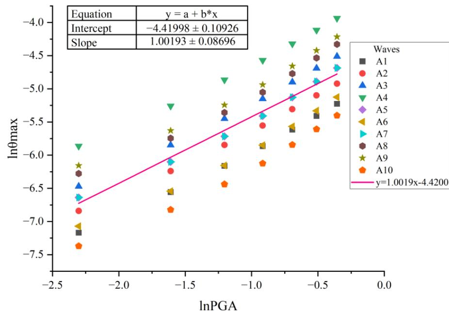
**Figure 4.** The fit of the  $\ln \theta_{max}$  to the  $\ln PGA$ .
