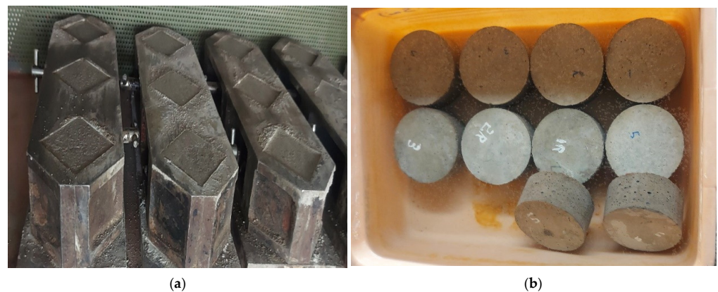
Figure 2. (a) Mortar cube molds. (b) Mortar cylindrical discs.
