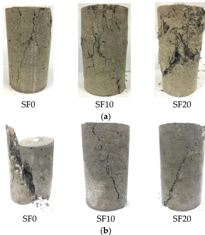
**Figure 16.** Typical failure modes of SFRC specimen under different confining pressures: (a) 0 and (b) 5 MPa.
