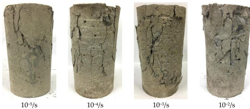
**Figure 15.** Typical failure modes of SF10 specimen with 0 MPa confining pressure at different strain rates.
