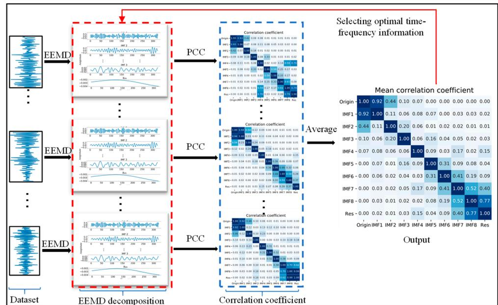
Figure 6. The procedure of optimal time-frequency selection.
