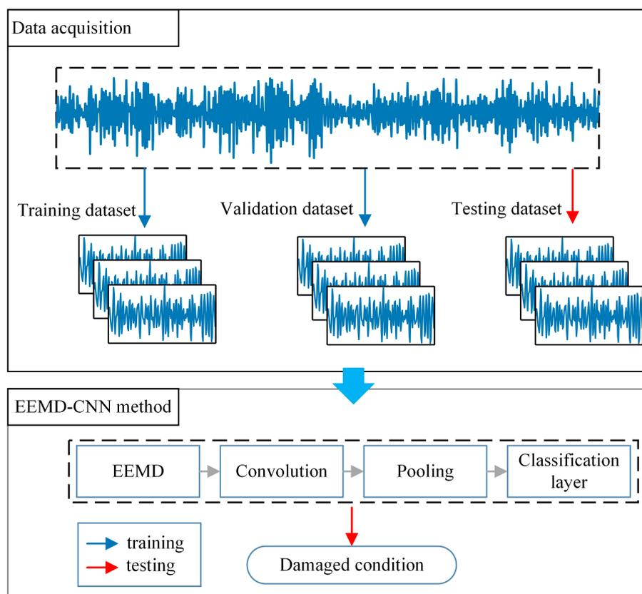
Figure 2. Flowchart of the proposed EEMD-PCC-CNN for structural damage identification.
