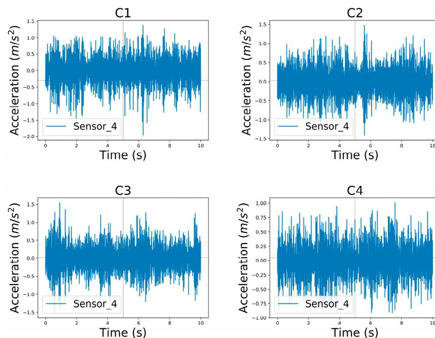
**Figure 4.** The acceleration curves on the three-story building structure.
