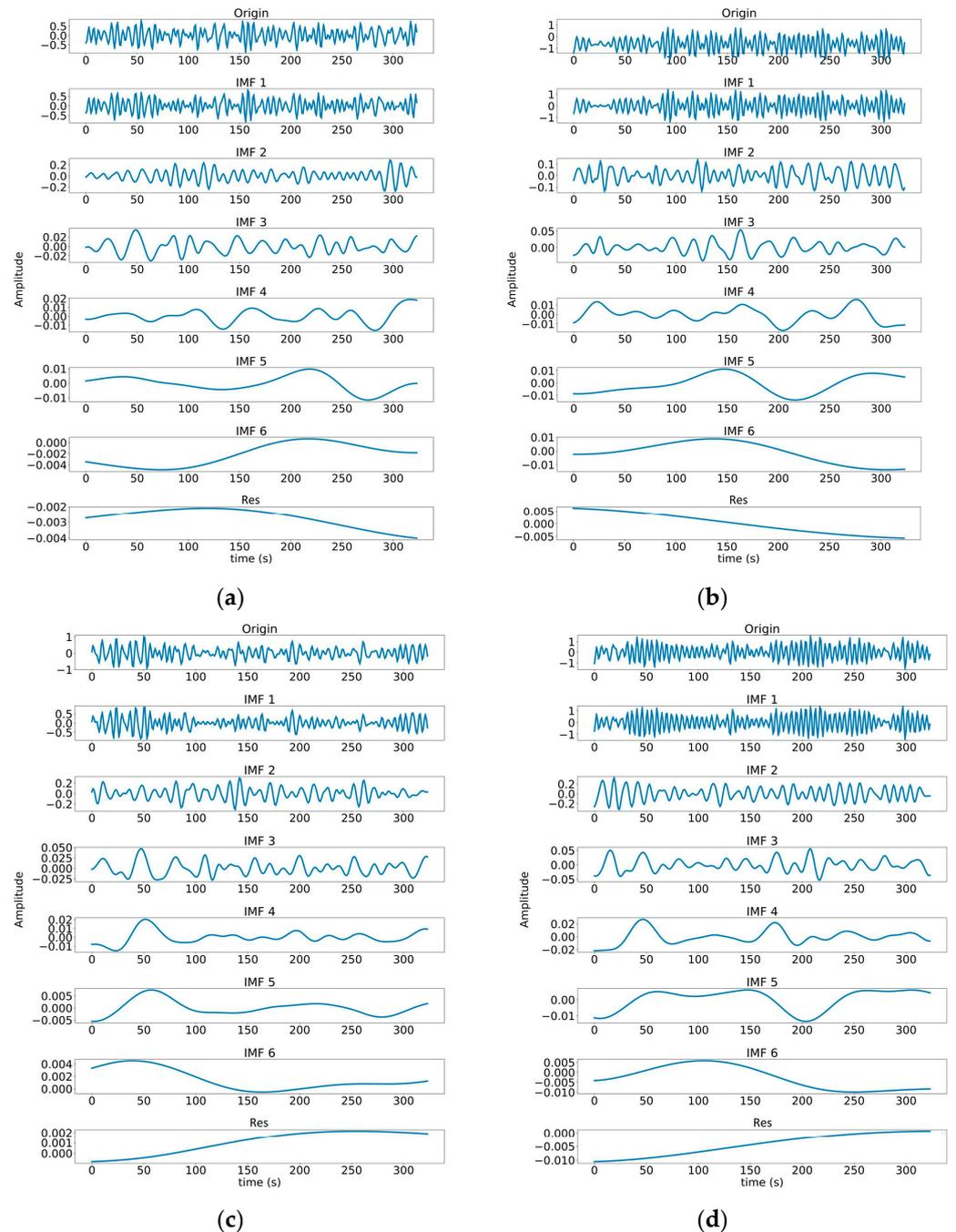
**Figure 5.** Results of EEMD decomposition of the accelerometer. (a) C1; (b) C2; (c) C3; (d) C4.
