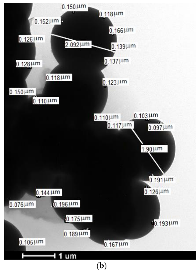
Figure 9. Trial-4 microcapsule TEM images at scales of (a) 500 nm and (b) 1 \mu\text{m} .
