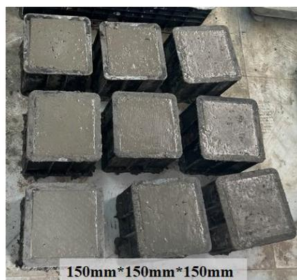
**Figure 1.** Concrete block.
