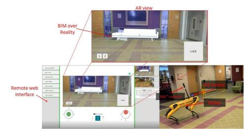
Figure 11. Experimental setup and user view in use case 1 experiment.
