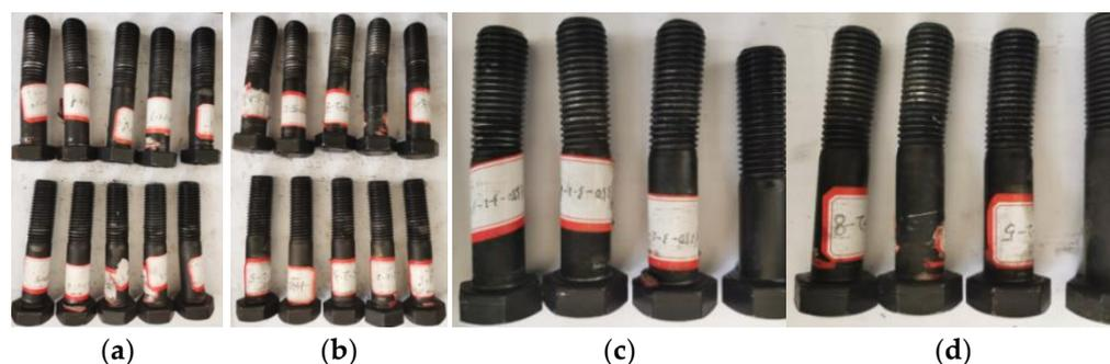
**Figure 11.** High-strength bolt of specimen: (a) H350-3-2 (b) H350-4-2; (c) Bending deformation of No. 1, 9 and No. 10 length bolts of H350-3-2; (d) Bending deformation of No. 5, No. 7 and No. 8 bolts of H350-4-2.
