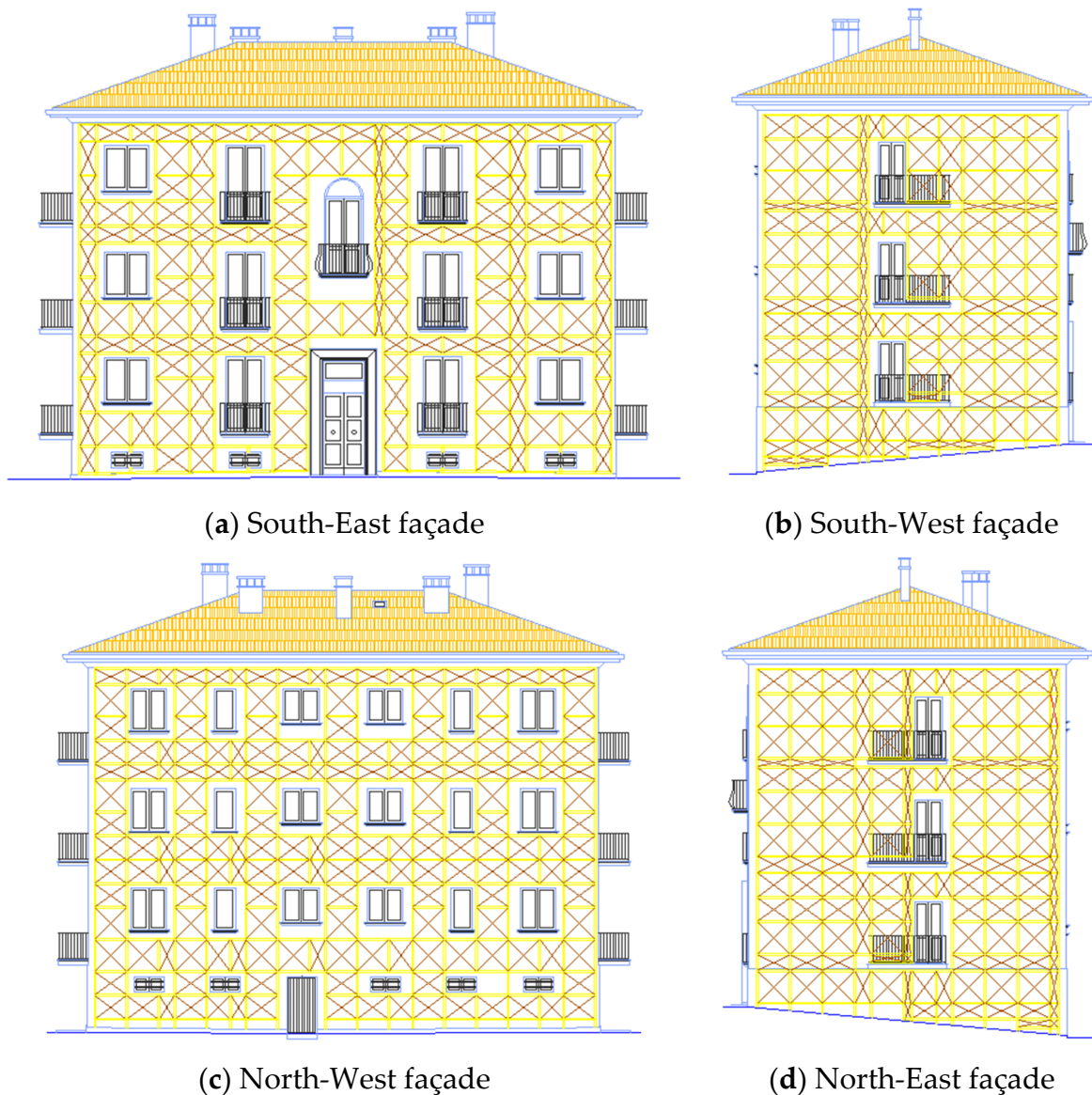
Figure 16. Application of the Resisto 5.9 coat system on the building facades (North-East (a), South-East (b), South-West (c) and North-West (d)).
