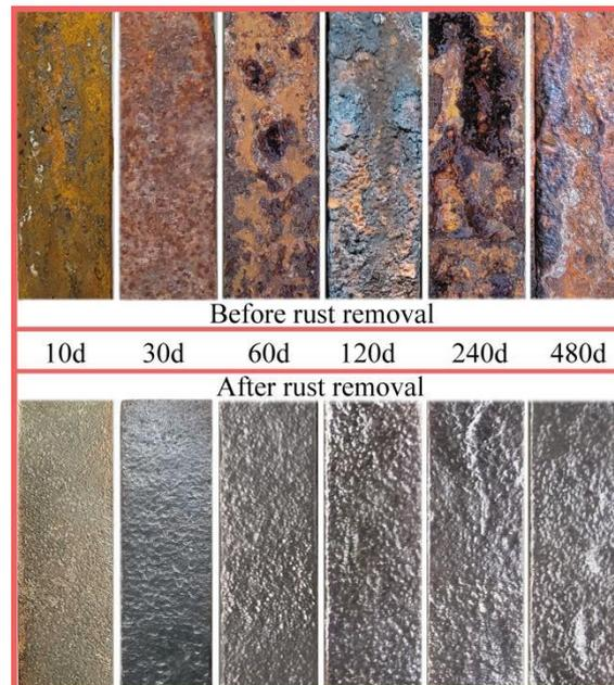
**Figure 1.** Corroded steel plates.
