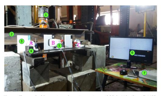
**Figure 7.** Photograph of the experimental setup in a specimen with labels. (1) Loading cell, (2) I-beam specimen, (3) grating panel, (4) linear guide (5) CCTV camera, (6) monitor for operating the camera, (7) DVR box, (A–C) camera positions.
