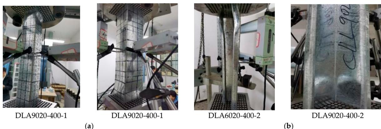
**Figure 10.** Buckling mode of short angle column with a length of 400 mm. (a) Local buckling. (b) Distortional buckling.
